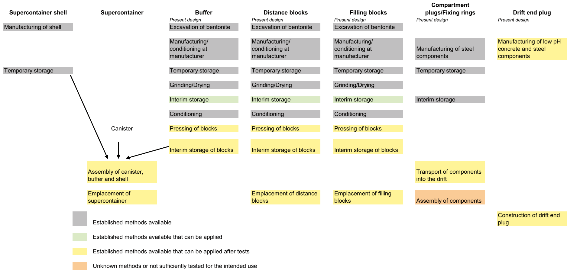
Figure 2-10. Production lines for supercontainer and auxiliary installations for KBS-3H and an estimate of the situation for technology development.
