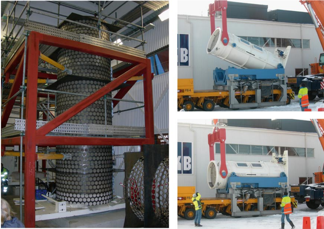
Figure 4-3. Left: Assembled supercontainer in the vertical position at Äspö. Right: The supercontainer is placed into a transport tube for transportation down to the underground test site at Äspö HRL.
