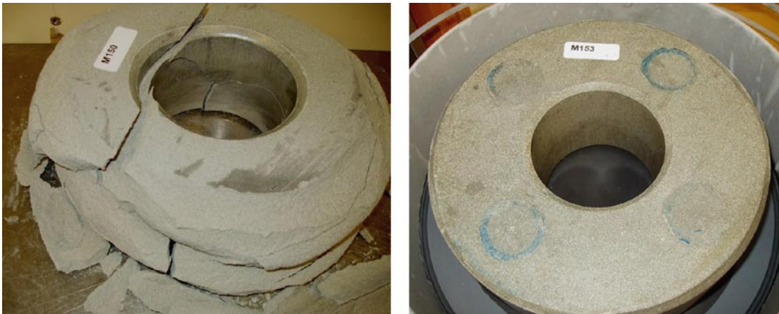
Figure 4-4. Example of cracking of buffer by humidity; block with low initial water content after 8 hours (left) and with high water content after 3 months (right) /Börgesson et al. 2008/.
