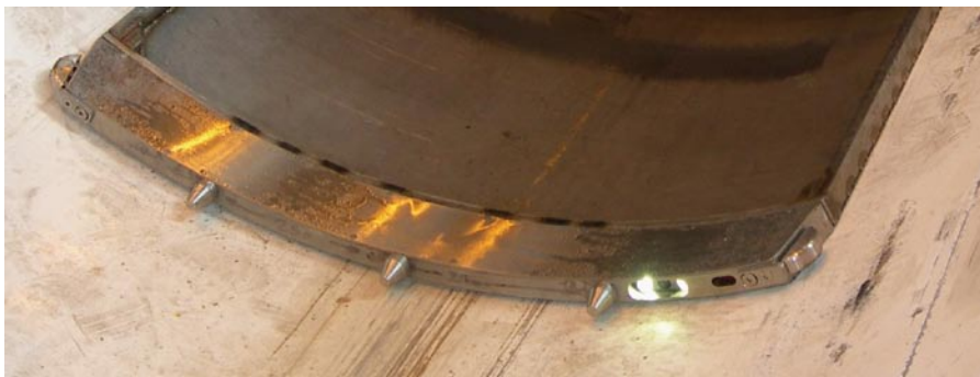
Figure 6-4. Front of slide plate with camera and lighting.
