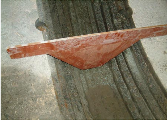
Figure 4-7. Template for verifying the shape of the slot for the compartment plug.
