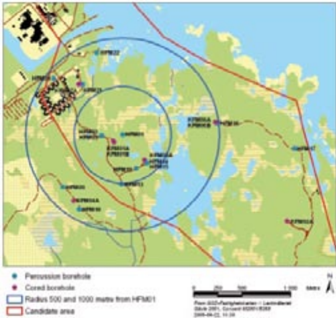
Figure 6-1. Map of tracer test configuration in relation to the Forsmark site investigation area. The positions of the boreholes included in the test are shown as well as areas corresponding to 500 m and 1,000 m radius (concentric circles) from HFM01. (Figure taken from /Wass and Andersson 2006/).
