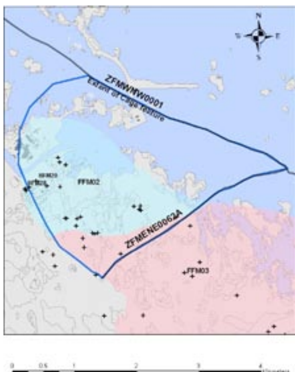
Figure 2-3. The hypothesised horizontal extent of the discrete features as described by /Follin et al. 2008/. The feature approximately covers fracture domain FFM02 and is thought to terminate against the Singö deformation zone to the north (ZFMWNW0001) and ENE0062A to the southeast. The crosses mark the positions of percussion and core-drilled boreholes for which transmissivity measurements are available.
