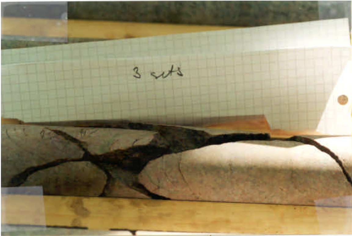
Photograph No. 4. Fractures of Set 2 with different dip direction
