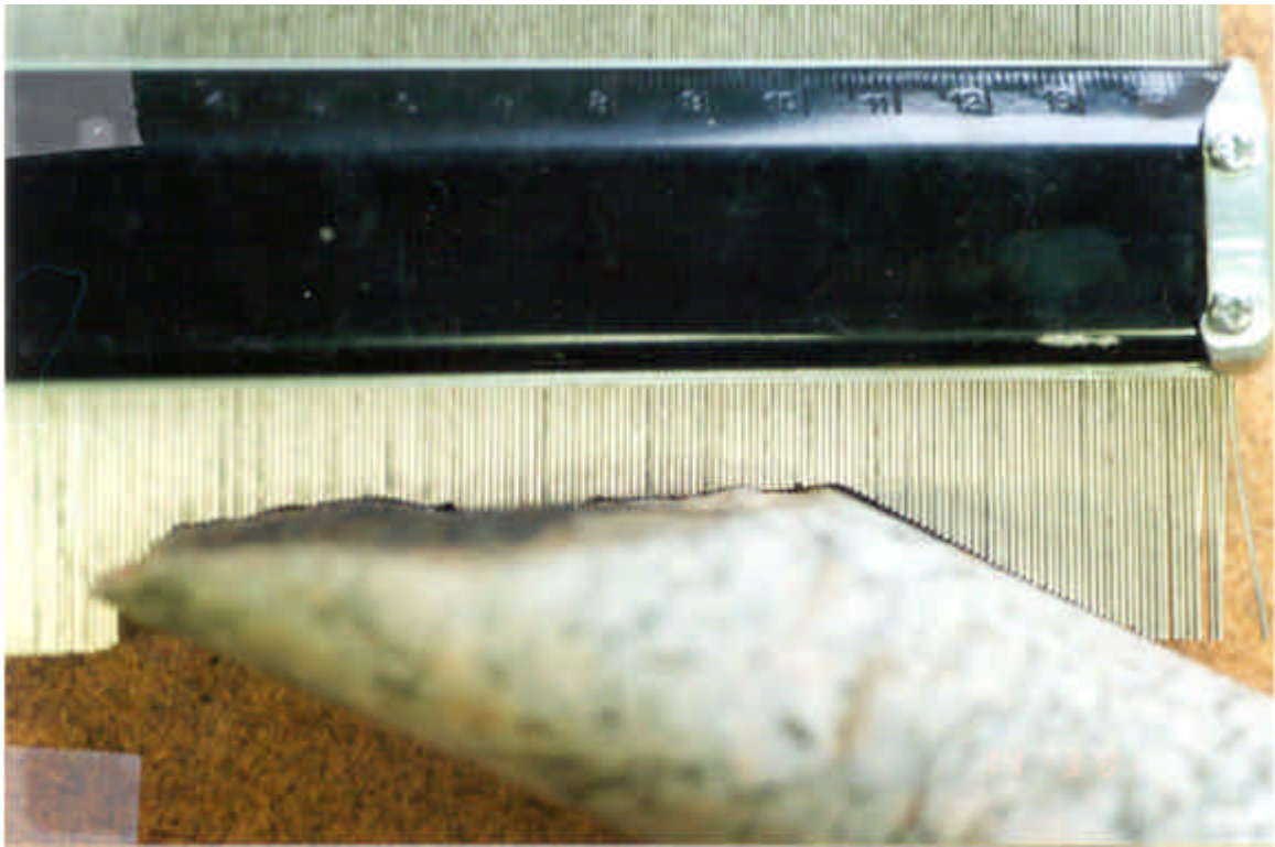
Photograph No. 3. Profiling by the use of profilometer
