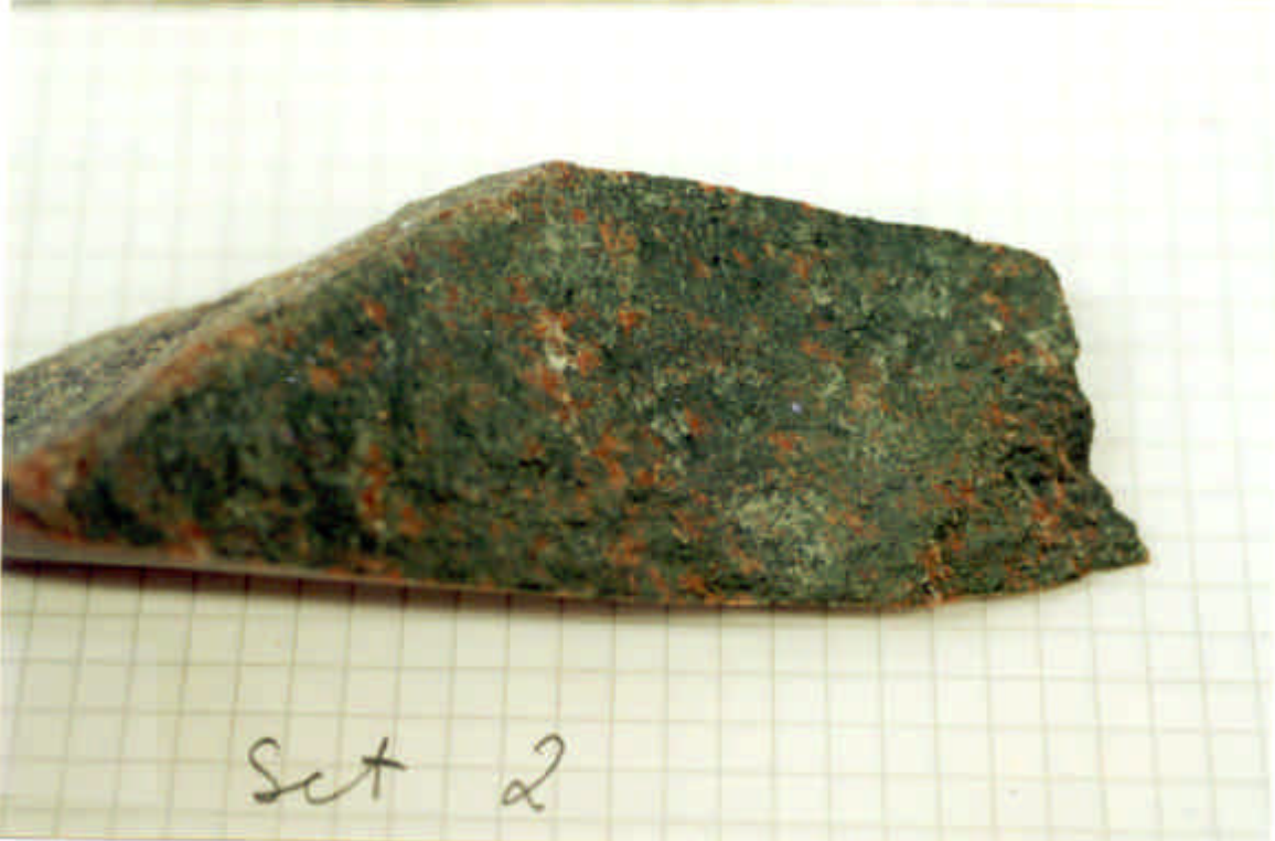
Photograph No. 5. Fracture with coating of chlorite and some calcite
