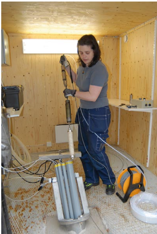
Figure 4-3. Lowering of equipment in the water stand-pipe in order to pump water from the borehole section. From the bottom; filter, small inflatable packer and pump.
