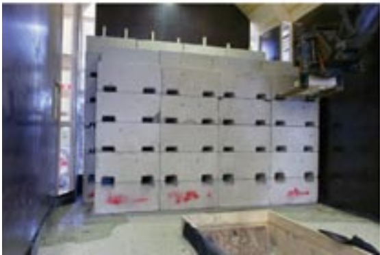
Figure 4-6. Stacking test with concrete blocks of relevant size and weight. Upper: Placement of blocks by use of the “Mecalac”. Lower: Concrete block masonries constructed with simultaneous measurement of joint apertures and time for installation.
