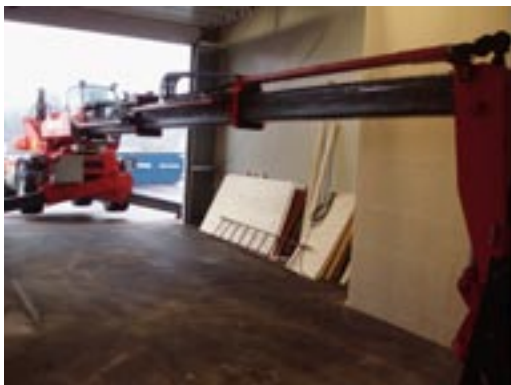
Figure 4-7. Testing of candidate tools for full-scale tests in the Bentonite Laboratory at Äspö. Left: Block stacking tests with telescope-type truck. Right: The “Gradall”, which is designed and used for ditching and other excavations.
