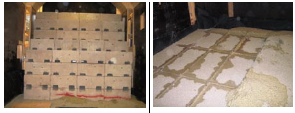
Figure 5-7 Left: After 10 minutes water came up from the water inlet positioned on the east side (0.25 l/min) and after additional 5 hours water could also be seen from the injection point in the middle. Right: After finishing the test it was observed that there were large dry parts under the blocks but the material under the joints was wetted.
