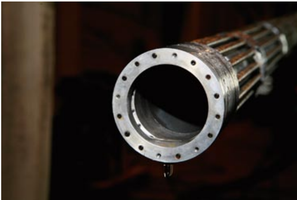
Figure 4-13. The picture shows the nozzle of the tube for blowing pellets with holes for adding water for reducing generation of dust.
