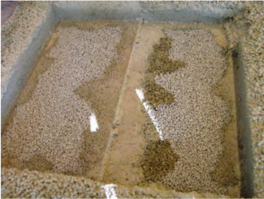
Figure 4-7 Picture showing the pellets after removal of the blocks. The pellets around the blocks had swelled quite a lot during the test time. Under the blocks there were large dry areas.
