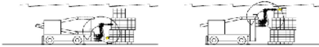
Figure 4-2. Stacking of the equally sized blocks. Placement of blocks by use of both robot arms to form three stepped units mutually displaced by \frac{1}{2} block length. The total length of each unit is 1.5 m.
