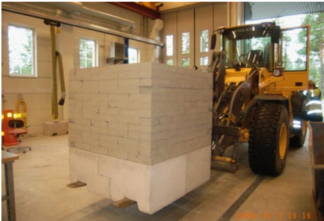
Figure 4-9. Testing of the stability of a module. Notice the bigger bottom blocks and layers of differently placed and oriented blocks.
