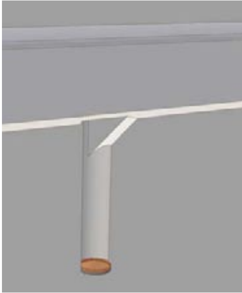
Figure 2-1. Deposition hole with bottom plate and ramp for making placement of the canister possible.
