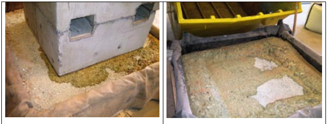
Figure 4-2 Left: Water from the injection point found a way up along the side and the continued saturation was done from the surface. Right: When finishing the test, dry areas were observed under the blocks. The surrounding bentonite had swelled up to a loose gel.
