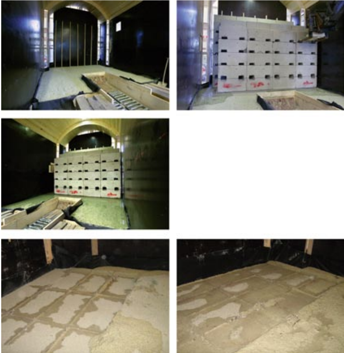
Figure 4-4. Examples of test arrangements for investigating of the impact of inflowing water on the settlement and bearing capacity of the foundation bed, as well as of the stability of block masonries.
