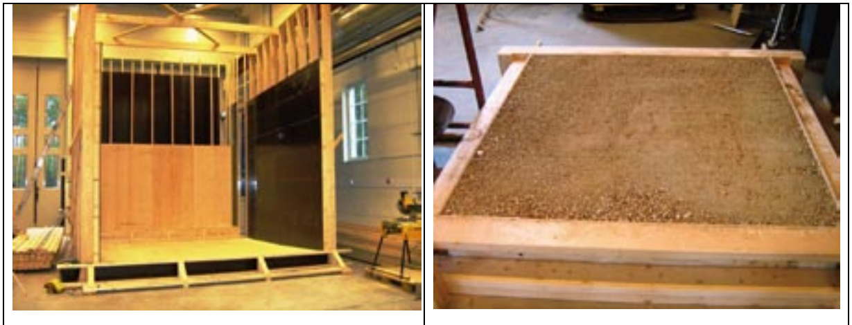
Figure 3-1 Left: An artificial tunnel part was built in the laboratory. Right: A special made box was used for testing of different compaction devices.
