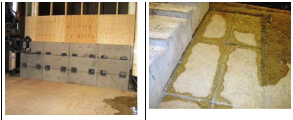
Figure 5-4 Left: After 10 minutes water came up from the water inlet positioned on the east side (0.25 l/min). Right: After finishing the test it was observed that there were large dry parts under the blocks but the material under the joints was wetted.
