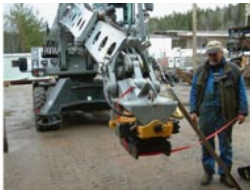
Figure 4-7. Testing of candidate tools for full-scale tests in the Bentonite Laboratory at Äspö. Left: Block stacking tests with telescope-type truck. Right: The “Gradall”, which is designed and used for ditching and other excavations.
