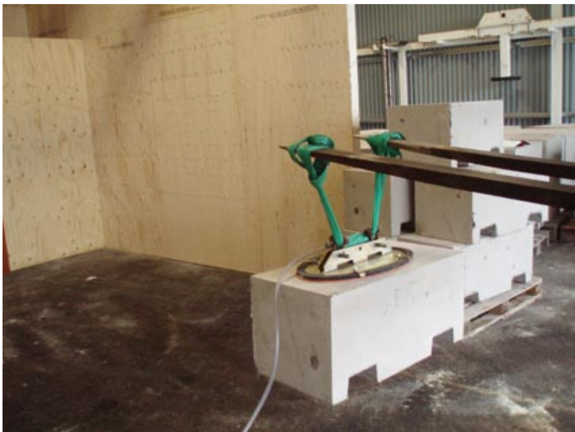
Figure 4-5. Vacuum plate for handling of concrete blocks.
