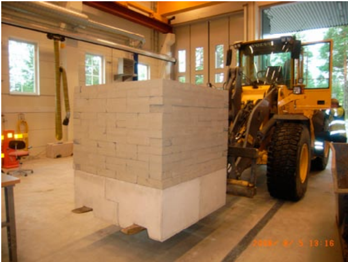
Figure 4-2. Test of the stability of a module.
