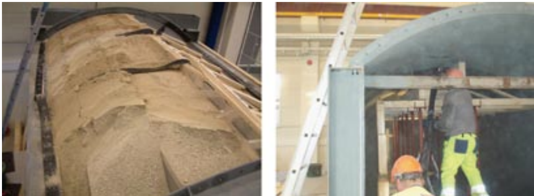
Figure 4-12. Arrangements in steel tunnel for filling tests using Minelco granulate.
