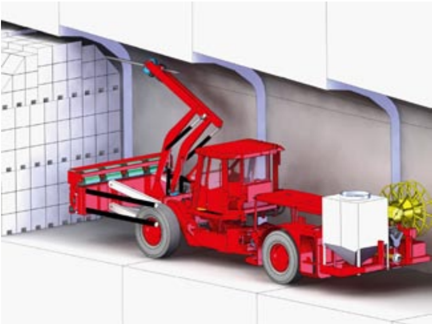
Figure 6-14. Pellet filling with the equipment placed closed to the steep block front.
