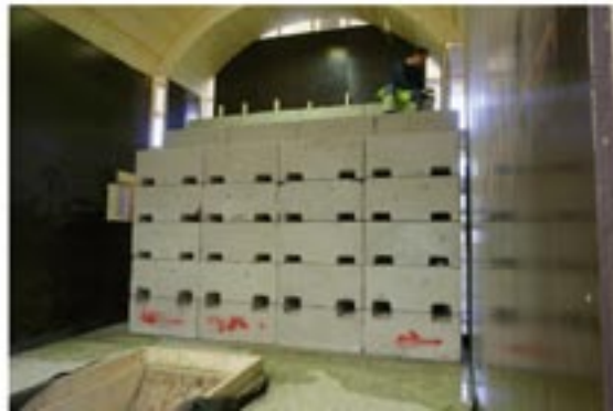
Figure 4-6. Stacking test with concrete blocks of relevant size and weight. Upper: Placement of blocks by use of the “Mecalac”. Lower: Concrete block masonries constructed with simultaneous measurement of joint apertures and time for installation.
