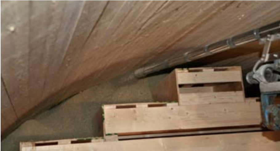
Figure 4-15. Pellet filling in the most narrow tunnel section.
