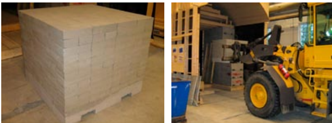
Figure 2-3. Stacking of the smaller blocks. Upper: design principle. Lower: example of full-scale test.
