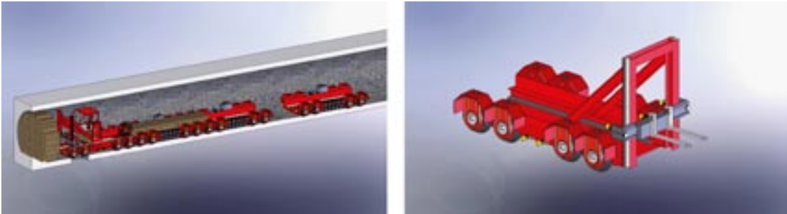
Figure 9-2. Backfilling of TBM-bored tunnels with “Module” method. Left: Set-out machines with magazine and delivery units. Right: Set.out machines (without cabin)
