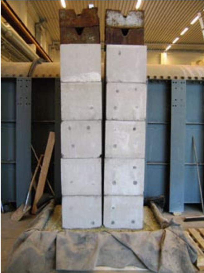
Figure 4-3 Picture showing the situation after 21 hours. The pile was very unstable and the gap between the blocks increased all the time.
