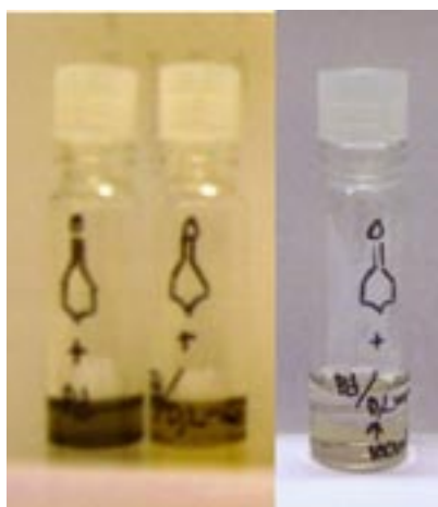
Figure 4-12. An organic phase consisting of cyclohexanone is left in contact with three different palladium containing aqueous phases (Left: 4.95 mM Pd, 0.81 M \text{NO}_3^- . Middle: 4.95 mM Pd, 3.3 mM D,L-methionine, 0.81 M \text{NO}_3^- . Right: 4.95 mM Pd, 60 mM D,L-methionine, 2M \text{NO}_3^- ) for 40 minutes.
