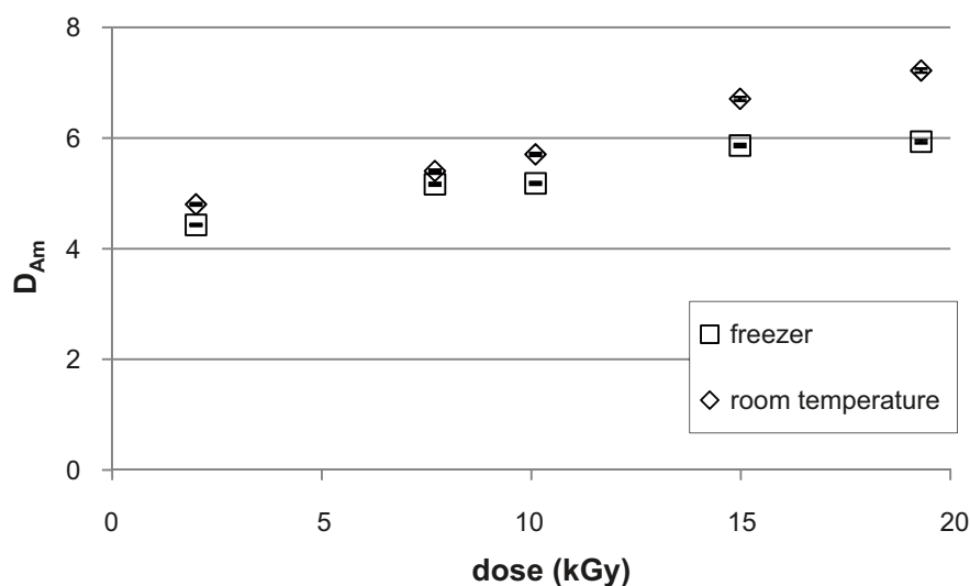
Figure 2-8. Distribution ratio ( A_m ) as a function of the dose received by the organic solvent before contact with the aqueous phase. The organic phase comprised 0.005 M CyMe 4 -BTBP in cyclohexanone and the aqueous phase comprised 0.01 M HNO 3 , 0.99 M NaNO 3 and traces of 241 Am and 152 Eu. The two series refer to temperature during the storage between irradiation and extraction experiments (4–5 months). In the freezer the temperature was around –25°C and the room temperature was around +21°C.
