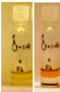
Figure 4-13. Cyclohexanone with 0.5 M of dioctyl sulfide is left in contact with 4.95 mM Pd in a solution with 0.81M nitrate concentration for 40 minutes (Left ) and 67 hours (right).
