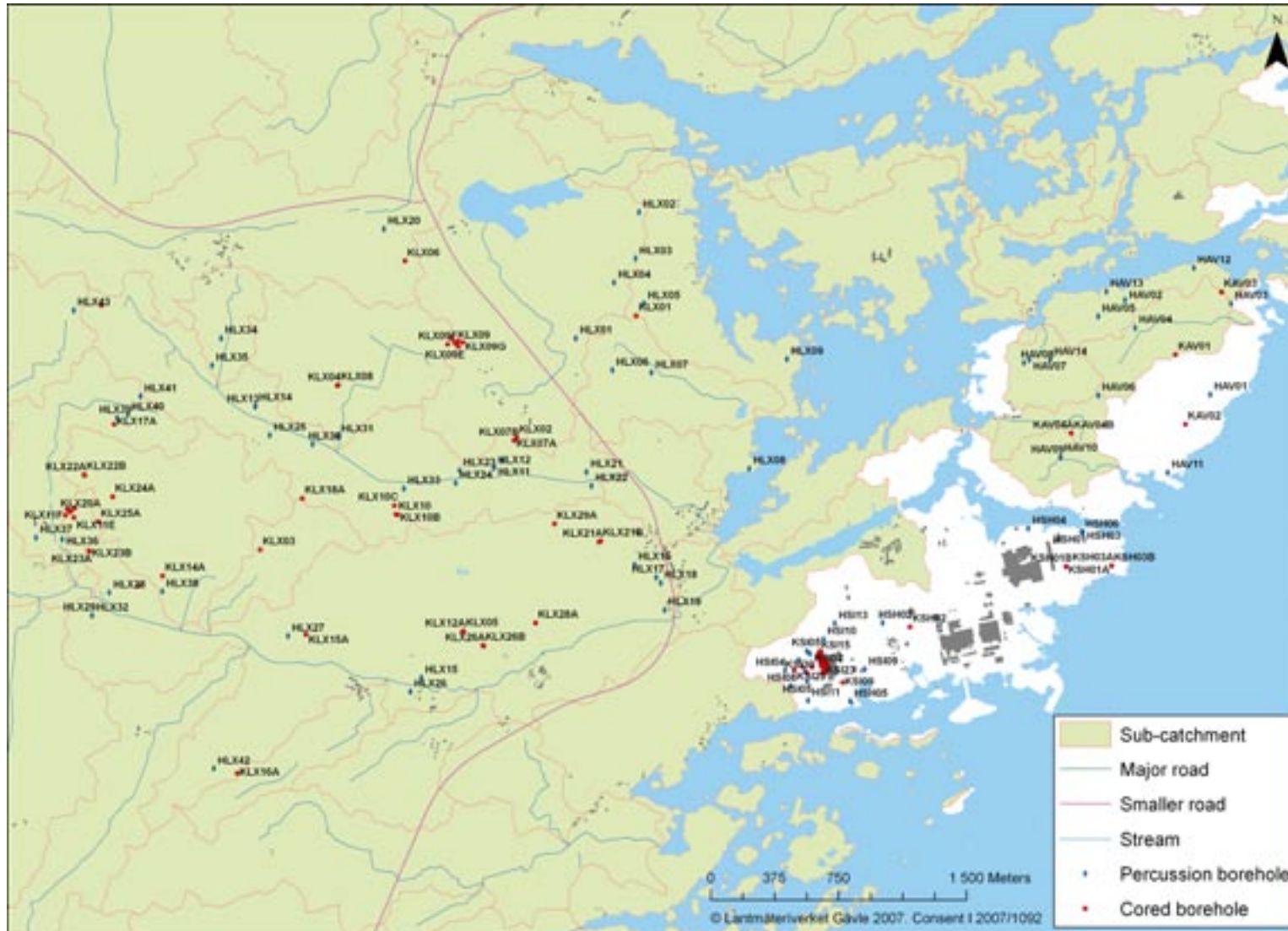
Figure 2-8. Groundwater sampling points in the bedrock in the Laxemar-Simpevarp area (cored- and percussion drilled boreholes).
