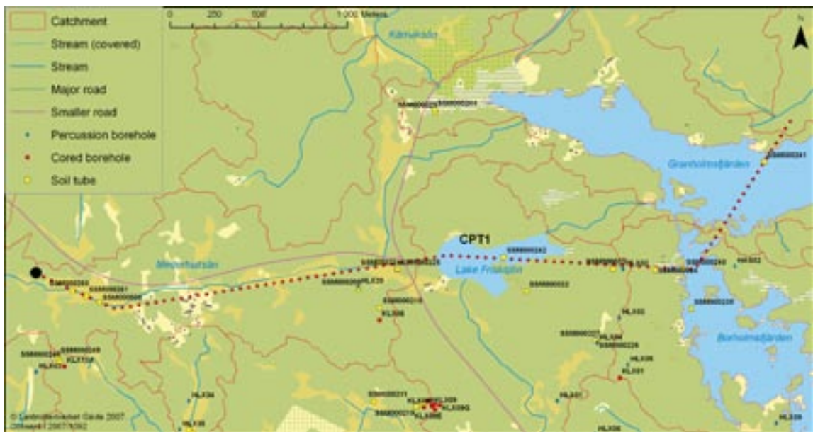
Figure 8-2. Map showing the location of the transect (denoted CPT1) in Figure 8-3 in relation to soil tubes, percussion boreholes and cored boreholes. The profile starts at the black dot at the left, and the three turns between the four sections are marked in Figure 8-3. See Figure 2-6 for a description of land use categories in the background map.
