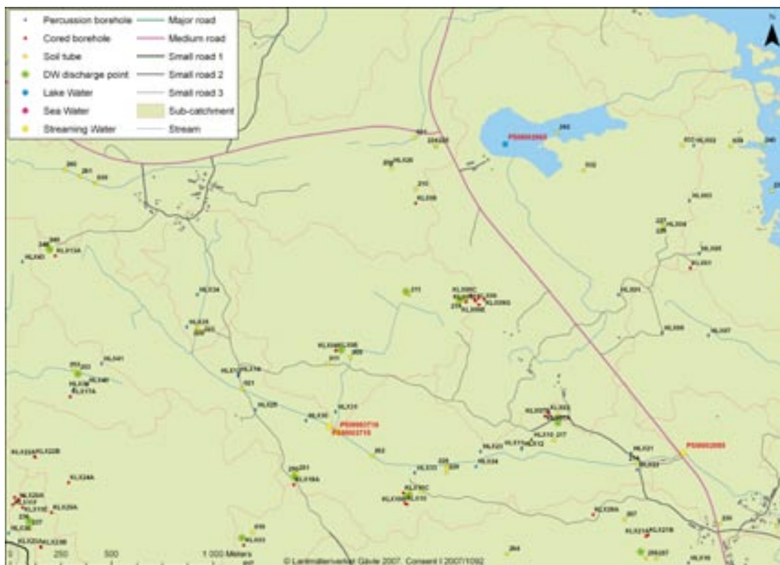
Figure 7-7. Close-up of the catchments of Lake Frisksjön (PSM002065) and the Ekerumsån River (PSM002085). Discharge points of flushing water from drilling of cored boreholes have also been marked in the map.
