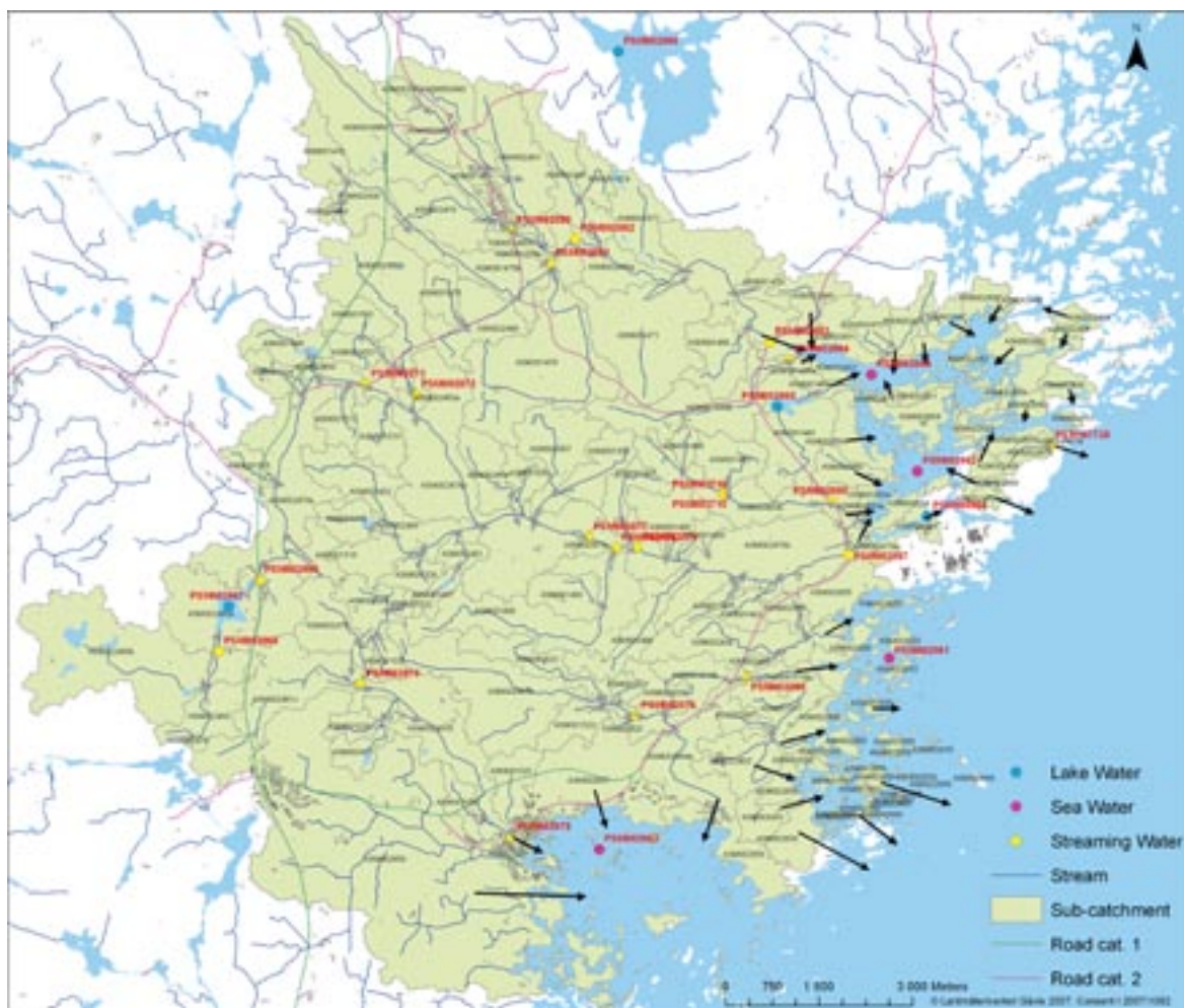
Figure 6-1. Sub-catchments and hydrological network of the Laxemar-Simpevarp area. Grey arrows show how sub-catchments (grey labels) are interconnected and black arrows show discharge to the Baltic Sea. Red labels indicate the locations of the hydrochemical sampling points. Several catchments are further divided into sub-catchments that intersect the hydrochemical sampling points (sub-catchments inherit the idcode from /Brunberg et al. 2004/ with addition of an additional letter at the end of the idcode, e.g. AFM002476a).
