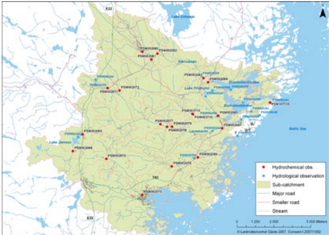
Figure 5-8. Location of hydrochemical stations in stream water (red) and hydrological observation points (blue) in the Laxemar-Simpevarp area. Among the hydrological observation points PSM000341, 343, 345, 347, 353, 364, 365 and 368 are surface water discharge measurement stations, PSM000342, 344, 348 and 359 are measurements of lake water level and PSM000369, 370 and 371 are observation points for sea water level.
