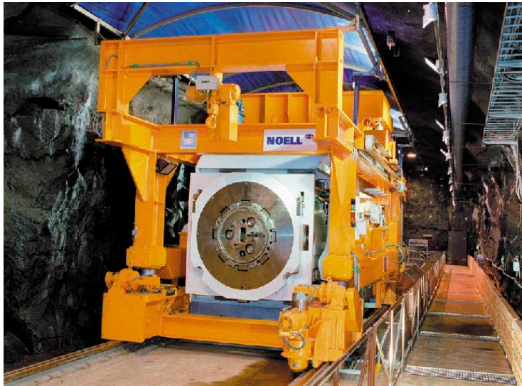
Figure 5. Deposition machine installed at Äspö Hard Rock Laboratory
