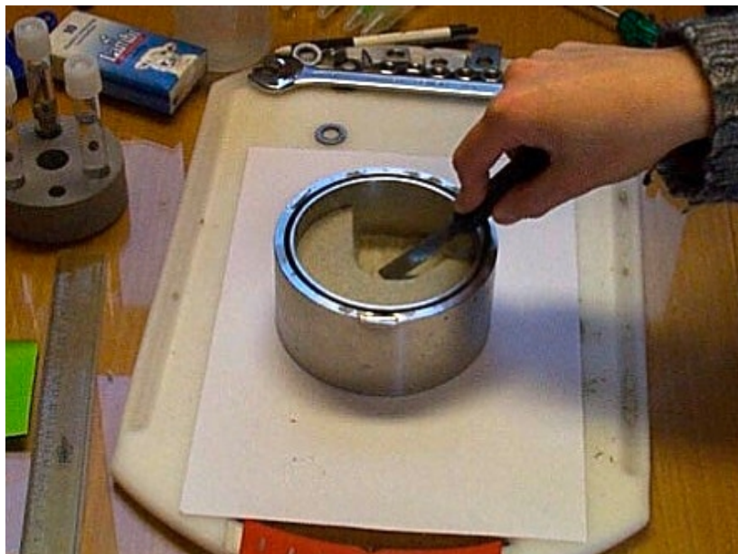
Figure 3-1. Cell in which clay powder was compacted. The lower picture shows the cell with lid and bottom plate removed and samples being extracted for determination of the water content distribution and for microstructural analyses after the water injection.
