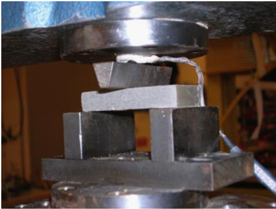
Figure 4-3. Test arrangement for determination of the tensile strength.
