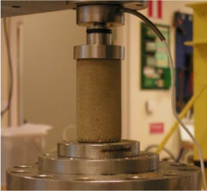
Figure 4-1. Test arrangement for determination of the shear strength of pre-compacted samples of backfill material.
