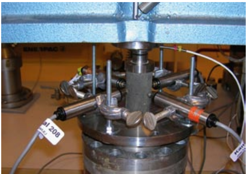
Figure 3-1. Test arrangement for determination of the Young's modulus and the Poisson ratio on pre-compacted backfill materials.
