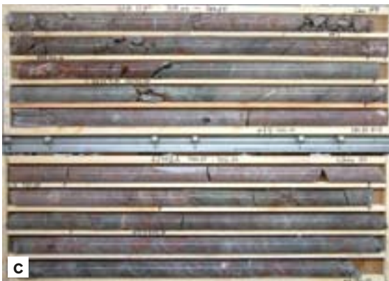
Figure 5-33. Character of deformation zones in the vertical or steeply dipping, WNW to NW set. a) Link to lineaments defined predominantly by magnetic minima connections that are concordant with the ductile structural grain in the bedrock. b) Crush zones, laumontite-sealed cataclasites and networks, and wall-rock alteration defined by dissemination of hematite and red staining, along part of a fault core interval in the Singö deformation zone (WNW0001) in borehole KFM11A (borehole interval c. 597 to 608 m). c) Cataclasite and fault breccia cut by younger fractures and networks sealed with quartz, calcite and other fracture minerals, along part of a pronounced fault core interval in the Forsmark deformation zone (WNW0004) in borehole KFM12A (borehole interval c. 315 to 326 m).
