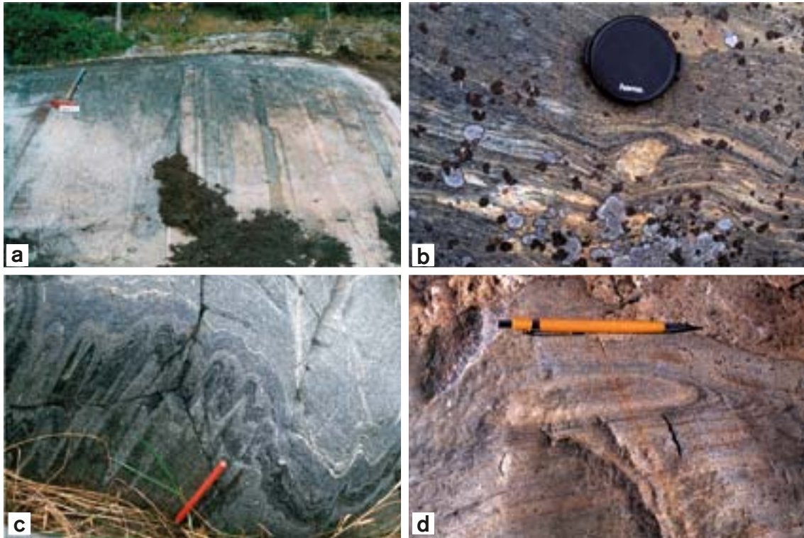
Figure 5-10. Character of the bedrock outside the Forsmark tectonic lens. a) Tectonically banded, foliated and lineated meta-igneous rocks close to drill site 4, south-west of the major synform inside the lens. b) Winged porphyroblast ( \delta -type) in rocks affected by high ductile strain close to SFR, to the north-east of the major synform inside the lens. A component of dextral strike-slip displacement is inferred. The highly strained rocks at this locality (PFM001235) are also folded. c) Folding of the highly-strained rocks at PFM001235. Folds of this type in this outcrop are dominated by S-asymmetry and are parasitic to the major synform. d) Eye-shaped, tubular fold in outcrop close to SFR.
