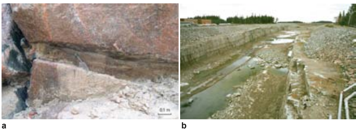
Figure 11-2. a) Laminated silt in an open fracture in the north-western part of the excavated area at drill site 5. The site was originally covered with till that has been removed. b) Horizontal fractures along the more than 1 km long canal between the Baltic Sea and the nuclear power reactors in Forsmark. These fractures are inferred to be sheet joints formed in connection with the release of stress in the bedrock.
