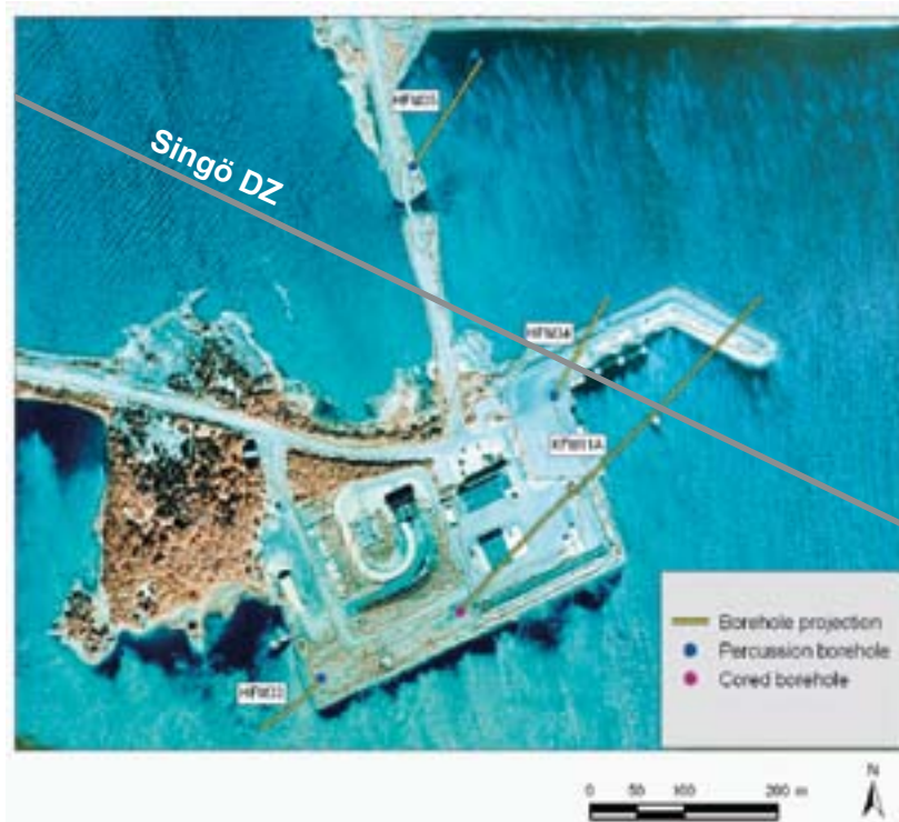
Figure 8-29. Map showing the SFR office buildings, the Singö deformation zones and borehole locations of HFM33, HFM34, HFM35 and KFM11.
