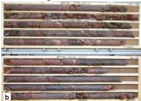
Figure 5-33. Character of deformation zones in the vertical or steeply dipping, WNW to NW set. a) Link to lineaments defined predominantly by magnetic minima connections that are concordant with the ductile structural grain in the bedrock. b) Crush zones, laumontite-sealed cataclasites and networks, and wall-rock alteration defined by dissemination of hematite and red staining, along part of a fault core interval in the Singö deformation zone (WNW0001) in borehole KFM11A (borehole interval c. 597 to 608 m). c) Cataclasite and fault breccia cut by younger fractures and networks sealed with quartz, calcite and other fracture minerals, along part of a pronounced fault core interval in the Forsmark deformation zone (WNW0004) in borehole KFM12A (borehole interval c. 315 to 326 m).
