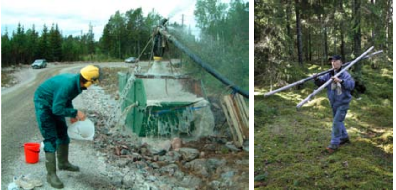
Figure 8-51. Two key features of the bedrock in the target area at Forsmark. Left: High water yields are often observed in the uppermost c. 150 m of the bedrock. Right: The large number of unbroken drill cores gathered at depth support the observation of few flowing test sections in the deeper bedrock.
