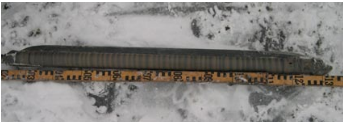
Figure 4-21. Example of a varved glacial clay collected in a small pond close to the Börstilåsen esker.
