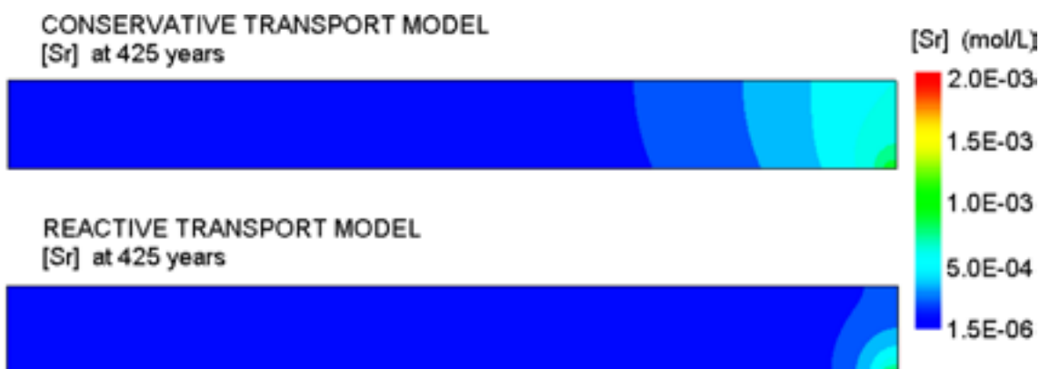
Figure 5-34. Comparison between the predicted strontium concentration in the modelled clay domain and the corresponding conservative transport case /Grandia et al. 2007/.
