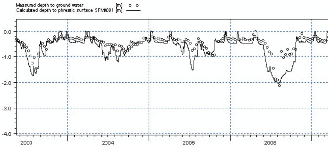
Figure 6-23. Calculated and observed depth to the groundwater table in SFM0001.
