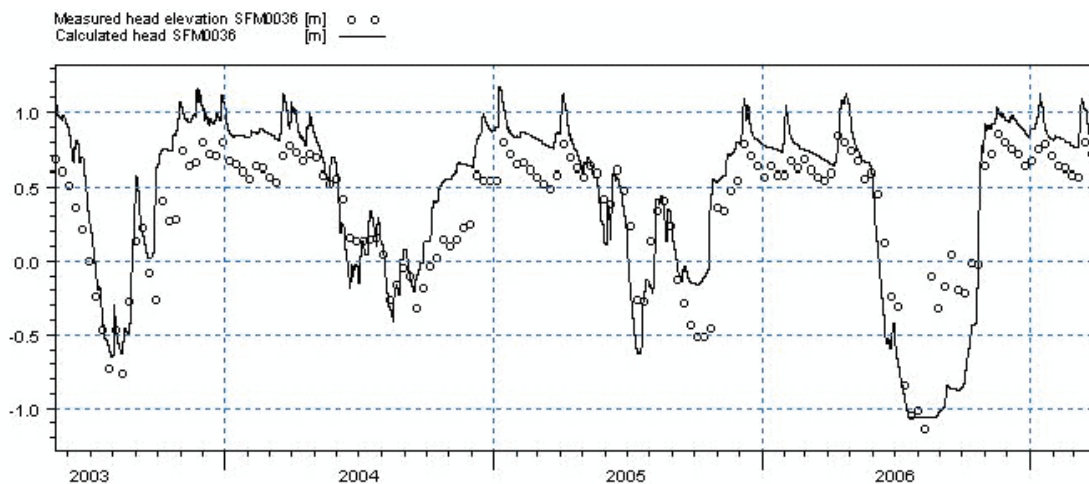
Figure 6-22. Calculated and observed groundwater head elevations in SFM0036.
