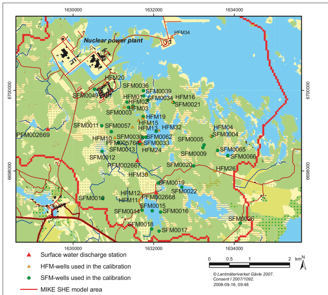
Figure 2-15. Positions of monitoring points used for model calibration and evaluation; SFM points are groundwater monitoring wells in QD and HFM points percussion-drilled boreholes in rock. PFM points are surface water discharge measurements. The red line indicates the boundary of the MIKE SHE model area.
