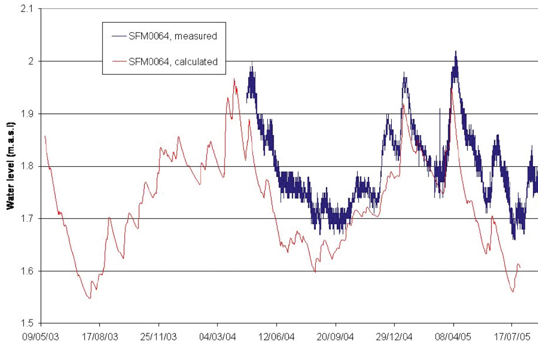
Figure 4-13. Calculated surface water level compared to measurements at station SFM0064 (Lake Gällsboträsket) from an early simulation.
