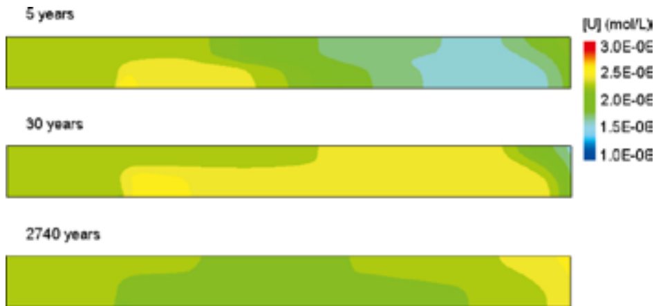
Figure 5-7. Predicted evolution of aqueous uranium in the modelled domain prior to repository release. At the initial 5 years, a transient plume of lower uranium concentration (light blue area) is predicted since deep groundwater has a lower uranium concentration than till porewater. Then, uranium is released into solution due to dissolution of \text{Fe}(\text{OH})_3 , leading to the higher concentration plume (yellow area). And finally, a balance between release of uranium into solution and adsorption of uranium on \text{Fe}(\text{OH})_3 is reached.
