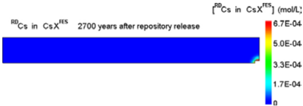
Figure 5-35. Concentration of ^{RD}Cs retained in FES of illite, at the end of the simulation period (2,700 years after repository release). Since caesium has a relatively high affinity for the FES, ^{RD}Cs is readily retained in the vicinity of the deep groundwater inflow point.
