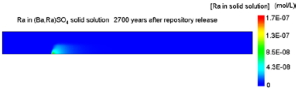
Figure 5-17. Predicted absolute concentration of Ra retained in (Ba,Ra)SO_4 solid solution, at the end of the simulation time (2,700 years after repository release). Ra is readily retained in the vicinity of the deep groundwater inflow point due to precipitation of (Ba,Ra)SO_4 solid solution.
