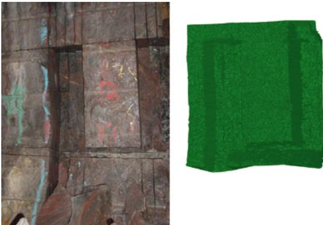
Figure 2-11. The investigated area, photo and mesh created from laser data.
