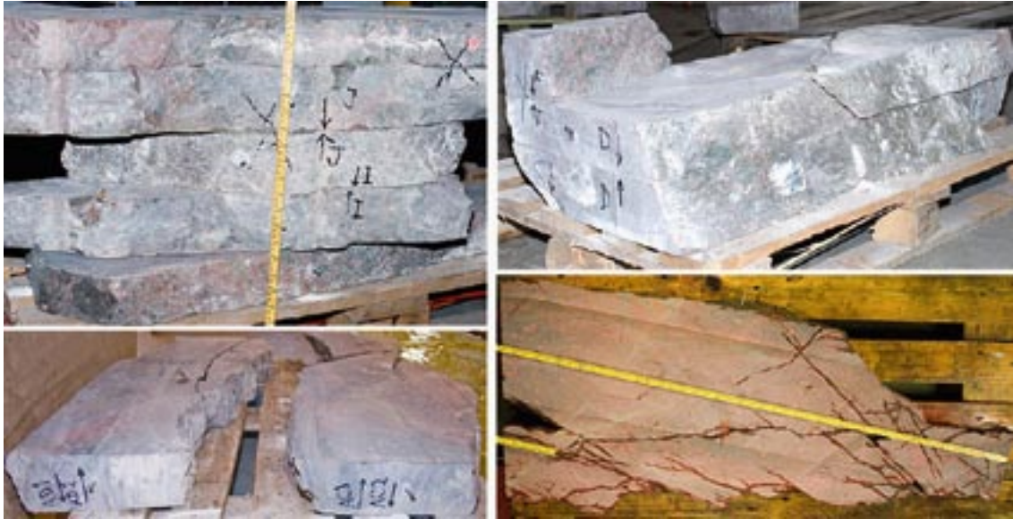
Figure 2-6. Pieces of the slabs.
