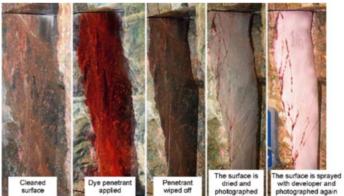
Figure 2-4. The different steps from washed surface to photographing.
