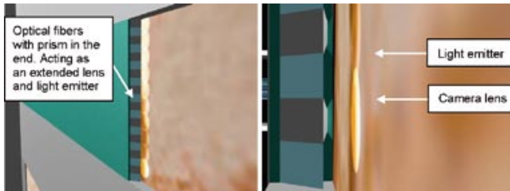
Figure 6-1. Hypothetical design of a scanning device showing the parts inside the slot.
