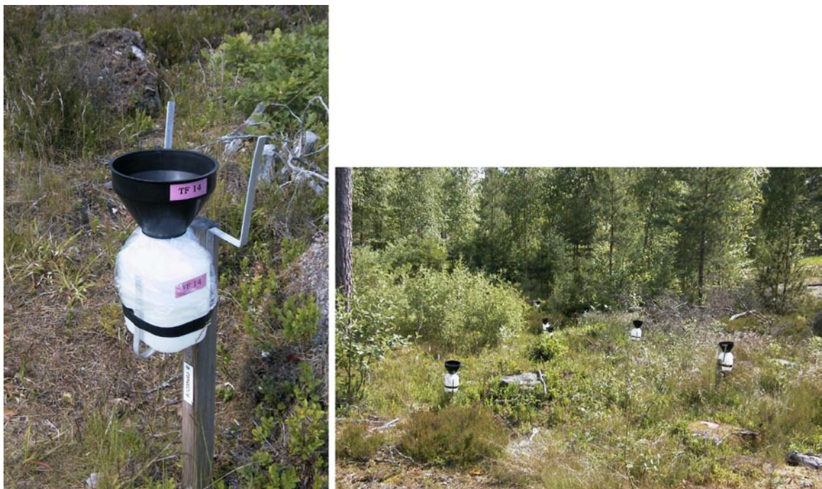
Figure 3 1. The samplers used in summer at the site for sampling of precipitation at the island of Äspö.
