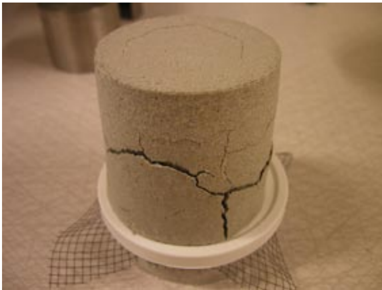
Figure 5-2. A 50 mm diameter cylindrical sample of compacted MX-80 bentonite after being exposed to humidity RH 100% for nine days (the photo is provided by Torbjörn Sandén/Clay Technology Lund Ab).
