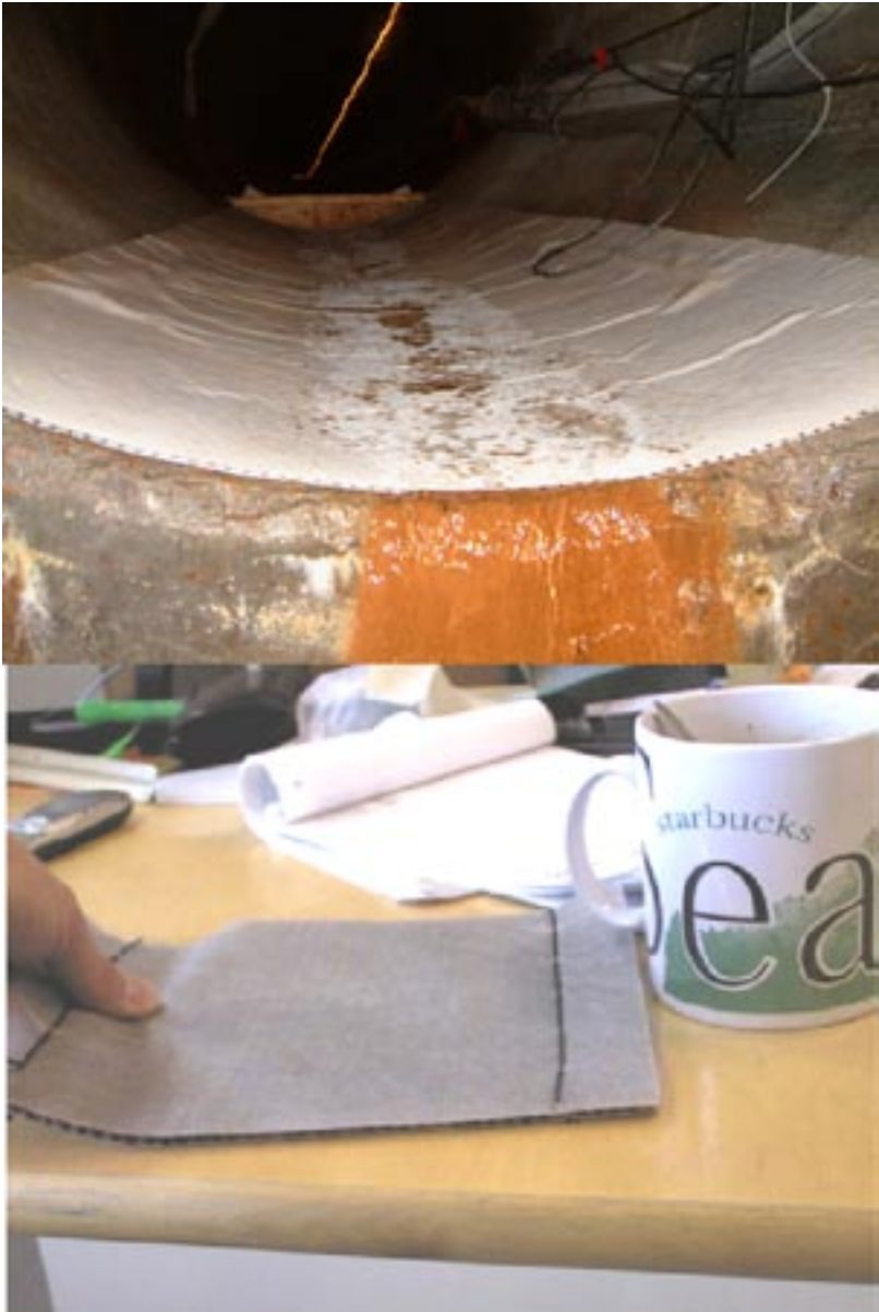
Figure 5-12. Enkadrain 5006H/T110PP drainage mat (above). The mat was tested at Äspö (top) and shall be covered with impermeable upper surface layer for the proposed use.
