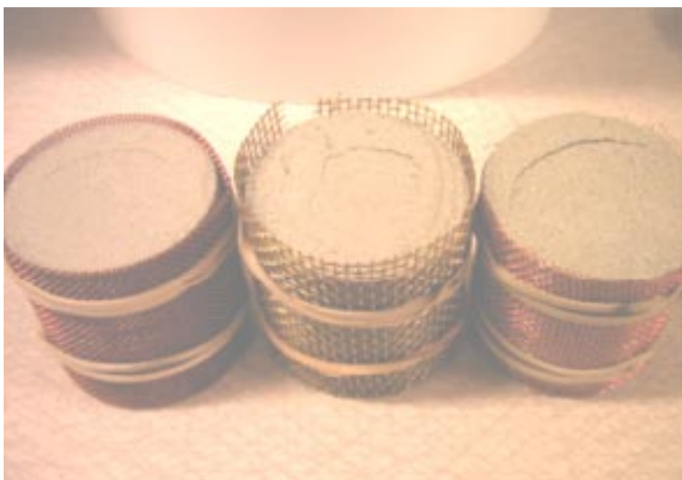
Figure 5-3. Example of three 50 mm diameter samples of bentonite wrapped in a mesh after being exposed to RH 100% humidity for nine days. Note: this small scale experiment does not show how distance blocks behave, however they give indications of certain processes related the interactions between mesh and bentonite (the photo is provided by Torbjörn Sandén/Clay Technology Lund Ab).
