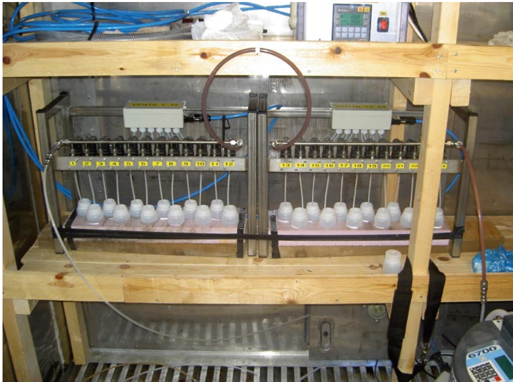
Figure 3-5. The automatic sampling equipment (24 magnetic valves) used at the withdrawal hole KFM02B.
