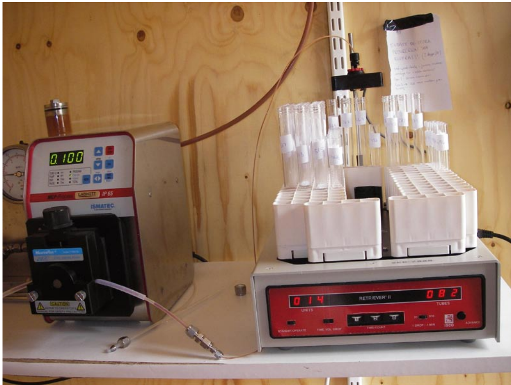
Figure 3-3. Peristaltic pump and fraction sampling equipment used at the injection hole KFM02A.
