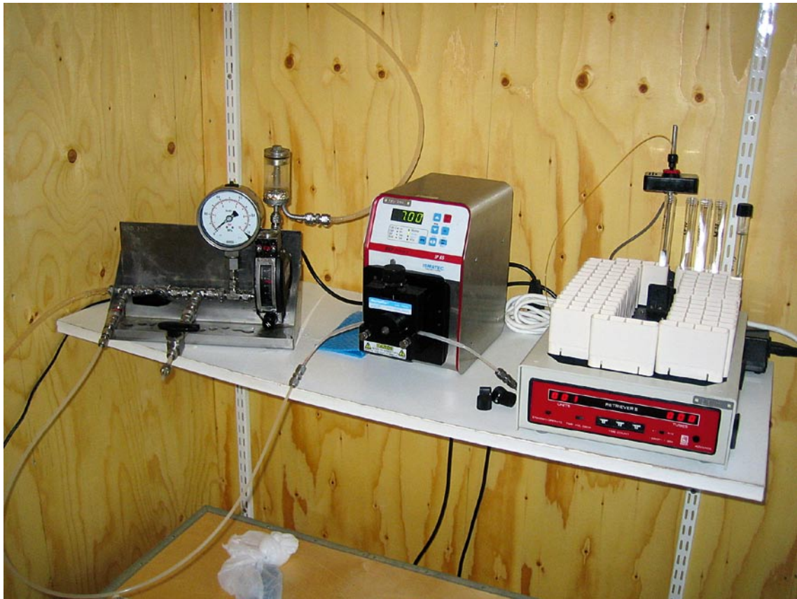
Figure 3-3. Circulation unit, peristaltic pump and fractional sampler used at the injection sections in the groundwater flow measurements and the tracer test.
