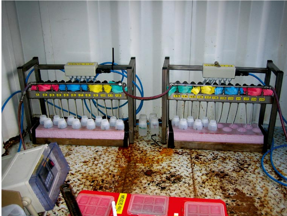
Figure 3-5. The automatic sampling equipment (24 magnetic valves) used at the withdrawal hole HFM14.
