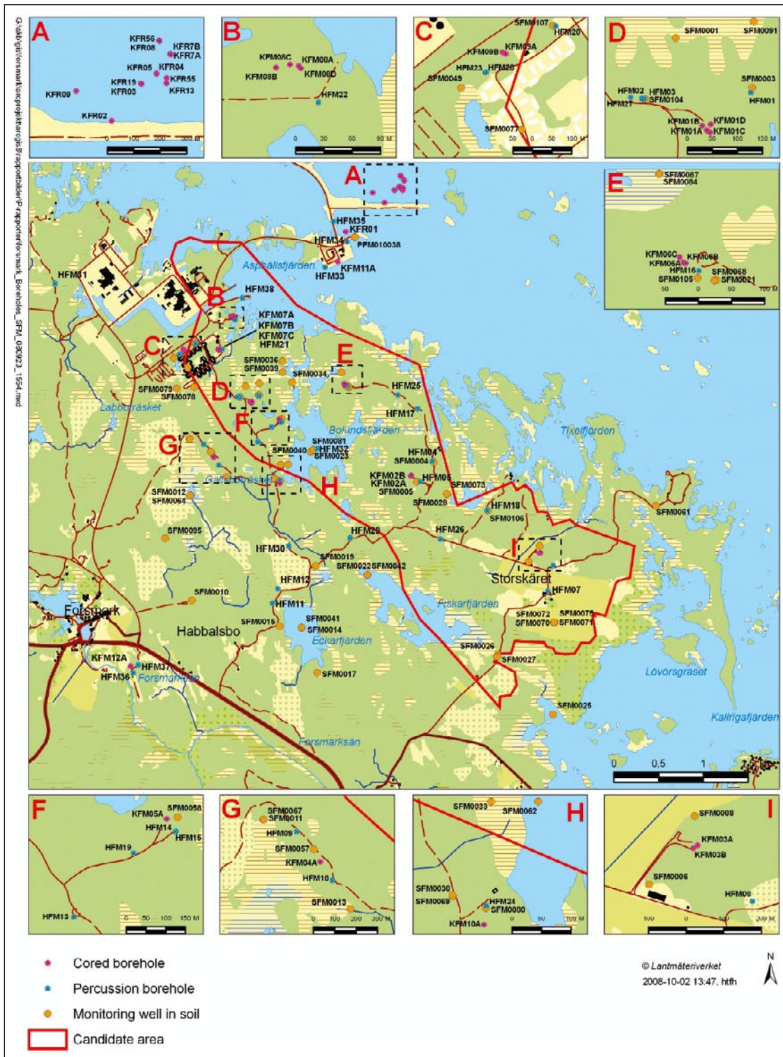
Figure 2-1. Overview of the Forsmark site investigation area with boreholes of different categories and surface water level gauges.
