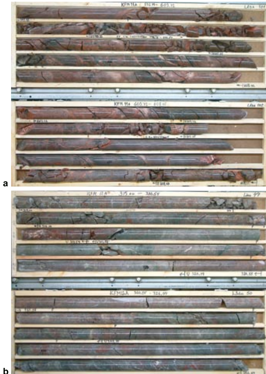
Figure 8-1. Character of fault core in the regionally important Singö and Forsmark deformation zones. a) Incohesive crush rock, laumontite-sealed cataclasites and networks, and wall-rock alteration defined by dissemination of hematite and red staining, along part of a fault core interval in the central part of the Singö deformation zone (ZFMWNW0001) in borehole KFM11A (borehole interval c. 597 to 608 m). b) Cataclasite and fault breccia cut by younger fractures and networks sealed with quartz, calcite and other fracture minerals, along part of a pronounced fault core interval in the central part of the Forsmark deformation zone (ZFMWNW0004) in borehole KFM12A (borehole interval c. 315 to 326 m)
