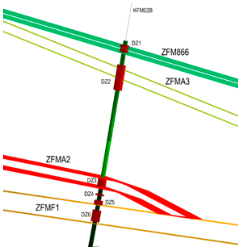
Figure 3-7. Prediction-outcome verification test for deformation zones along borehole KFM02B. Modelled deformation zones stage 2.2 (ZFM) compared with the six possible deformation zones in the single-hole interpretation (red cylinders). The orientation of the fractures along DZ4 and the geometric relationships shown in the figure argue against a correlation between this possible zone and the zones included in model stage 2.2. The length of borehole KFM02B is c. 573 m. See text for further discussion.
