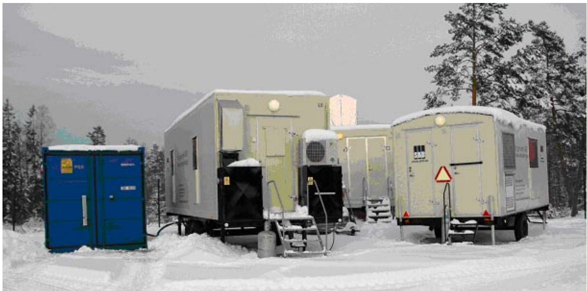
Figure 4-1. The mobile units used at KLX08; from left container for collecting the water from the borehole, laboratory unit, hose unit with downhole equipment and a unit for computer work.
