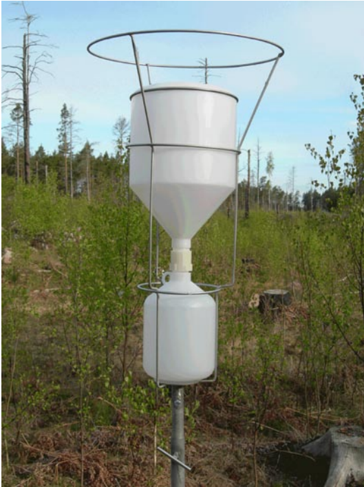
Figure 3-2. The new precipitation samplers (summer setup) used from May 2007 at Forsmark. Two sampler setups were used in order to increase the collected volume of precipitation.
