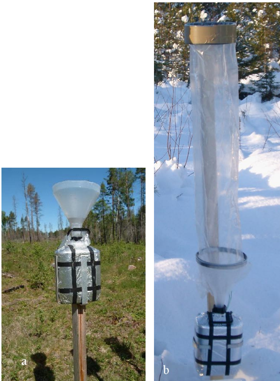
Figure 3-1. a) One out of five summer setups of the precipitations samplers used until April 2007. Five setups were used in order to increase the collected sample volume. b) One out of five winter setups of the precipitations samplers used until April 2007.
