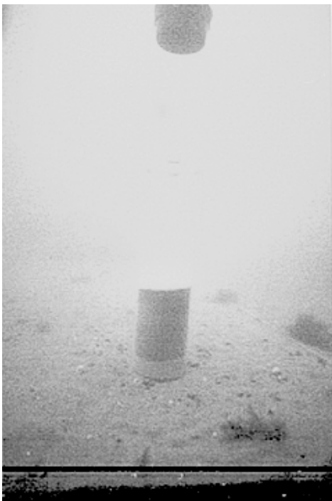
Photo no.1 Sediment cores from station no.3, 10.8 m depth. The redox-zone can be seen, especially in the middle core.
