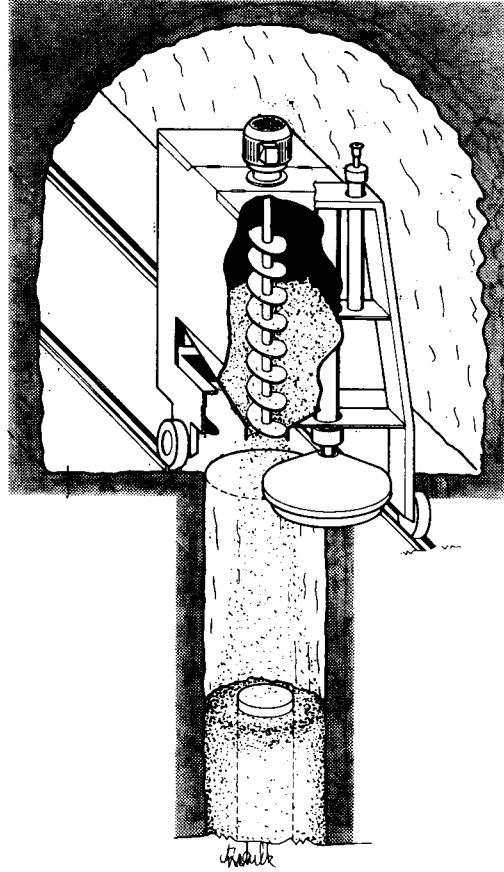
Backfill with buffer material
