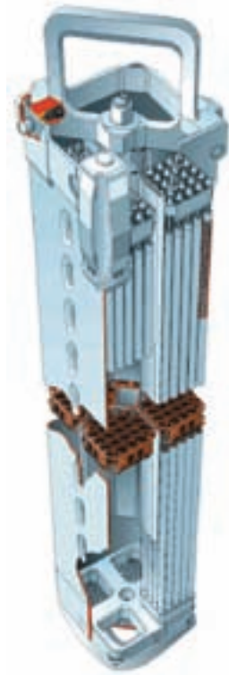
Figure 2-1. Fuel assembly of type SVEA 96.
