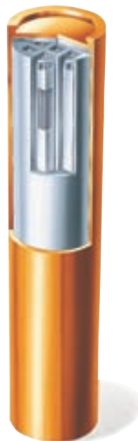
Figure 3-5. Design of canister shell and insert.
