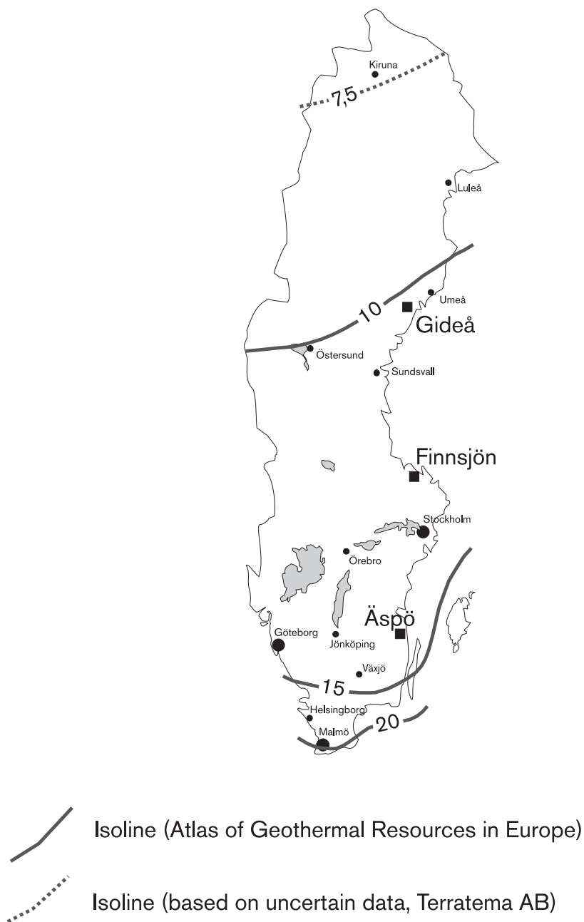
Figure 4-20. Temperature at 500 m depth in Sweden /after Sundberg, 1995/.
