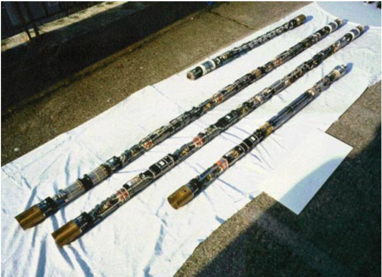
Figure 3-2. Photograph of the CHEMLAB probe sections. The entire length of the probe is 14 metres. The different sections are coated with steel tubes which are tightly connected to each other.
