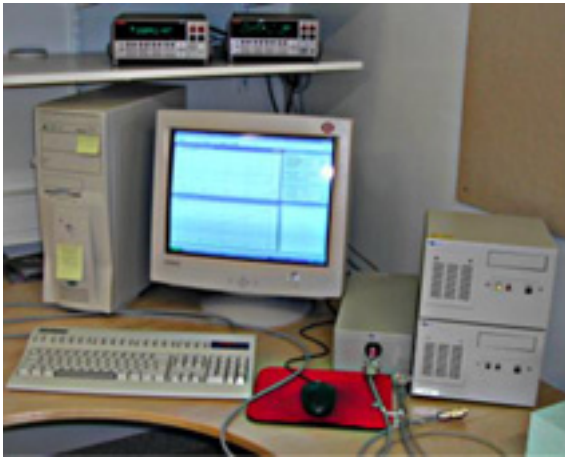
Figure 3-2. TPS-apparatus with source meter, multi-meter, bridge, and computer.
