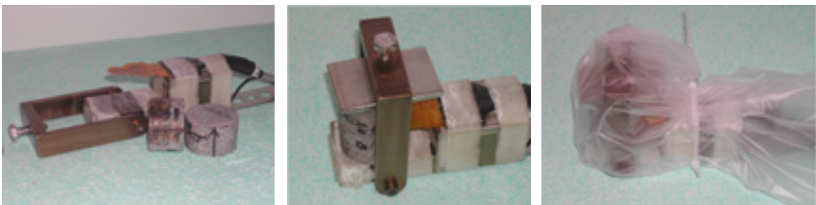
Figure 3-3. Specimens prior to mounting (left), mounted in stainless sample holder (middle), and sample holder with mounted specimens wrapped in plastic (right).
