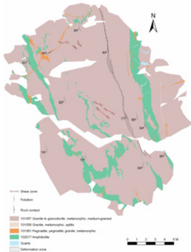
Figure 2-1. Besides the occurring rock types, the direction of the foliation and the position of a deformation zone cutting the outcrop along an approximately North-South direction as well as shear zones were observed.
