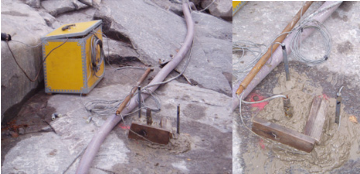
Figure 2. Logger, thermistors, and heat probe installed at location HFM95.
