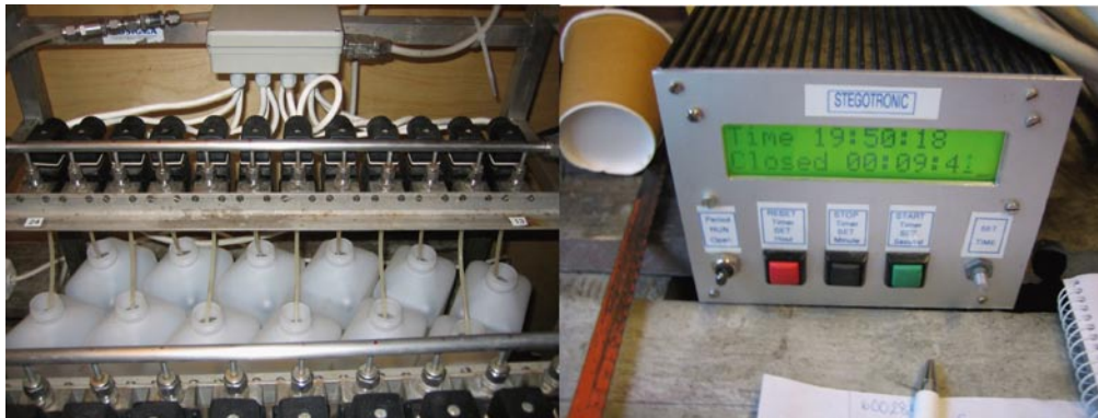
Figure 4-3. The automatic programmable sampler; magnetic valves (left) and control unit (right) (previous version to the one used in the test).
