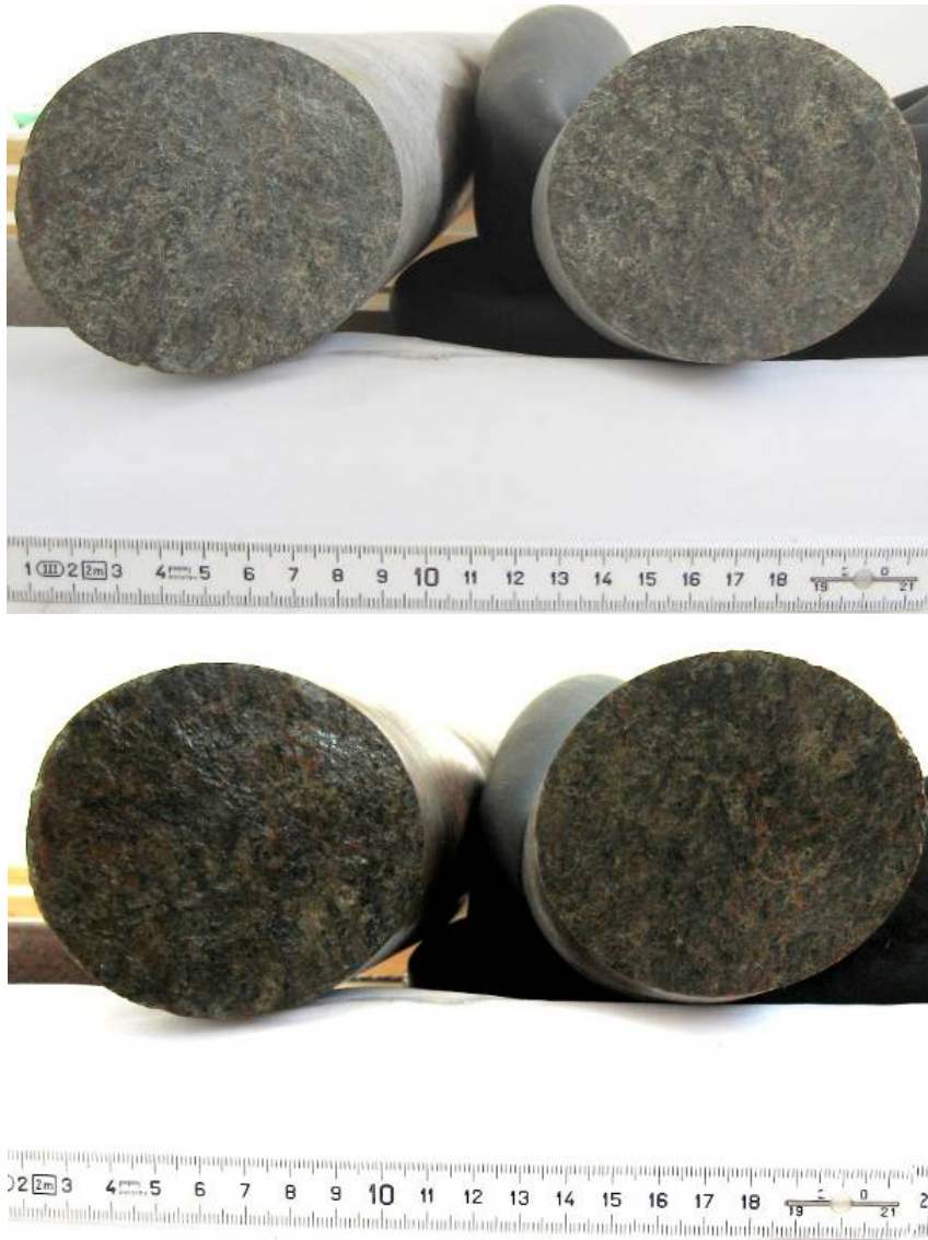
Figure 5–15. The fracture surface for the fracture at 1.327 m in the core. Dry and wet surface.
