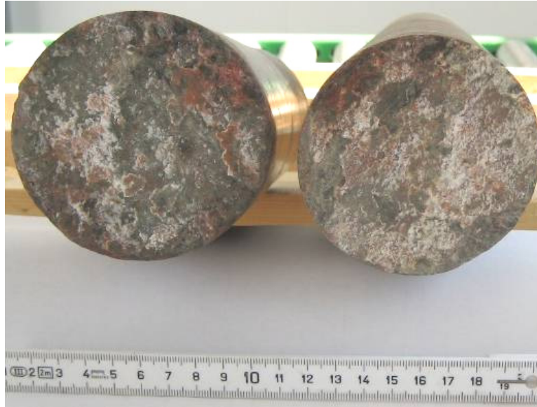
Figure 5–11. The fracture surface at 0.248 m from the core in dry condition.
