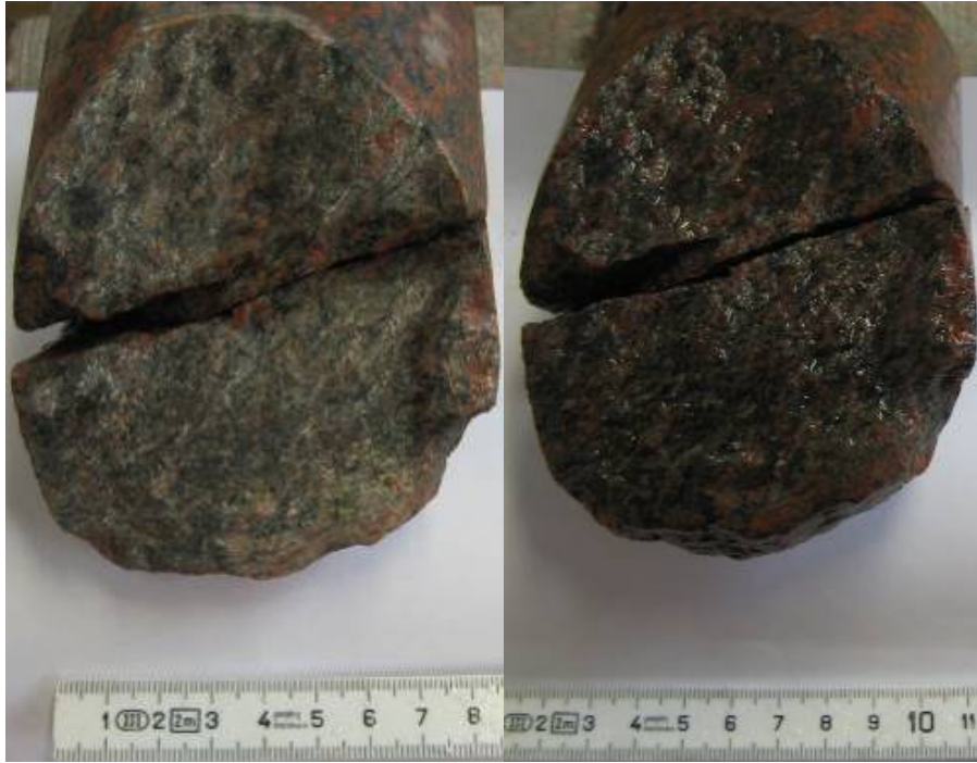
Figure 5–27. The fracture surface for the fracture at 0.394 m in the core. Dry and wet surface.
