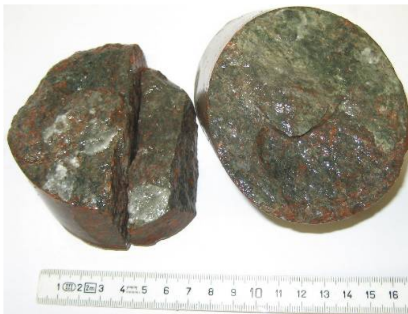
Figure 5–20. The fracture surface for the fracture at 0.734 m in the core. Wet surface.
