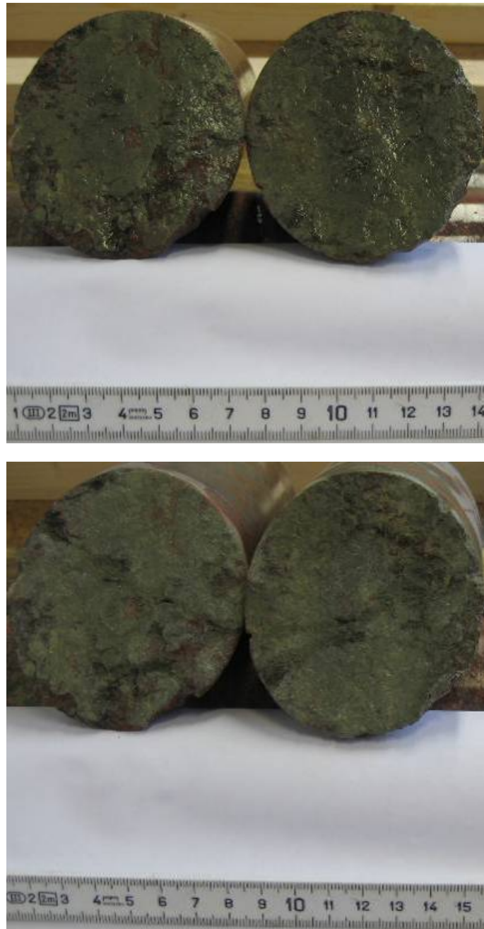
Figure 5–18. The fracture surface for the fracture at 0.592 m in the core. Dry and wet surface.
