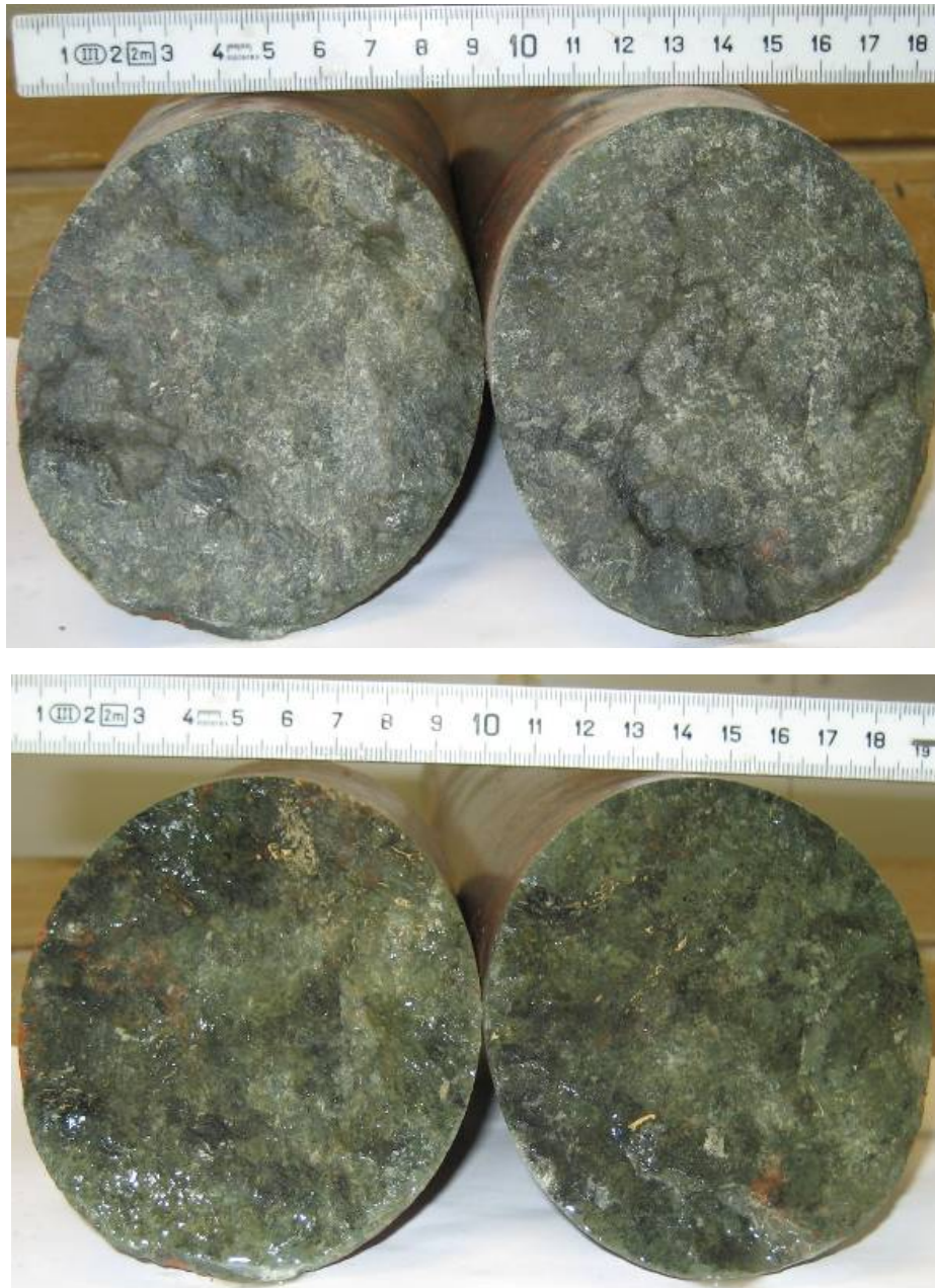
Figure 5–22. The fracture surface for the fracture at 1.212 m in the core. Dry and wet surface.
