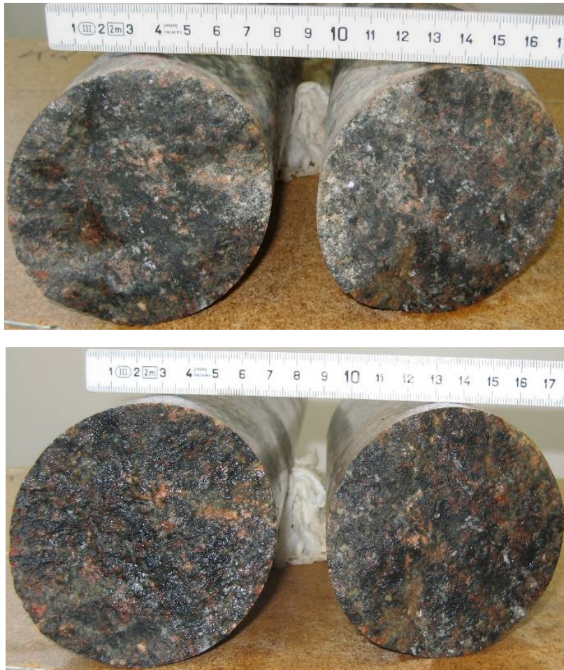
Figure 5–35. The fracture surface for the fracture at 0.14 m in the core. Dry and wet surface.
