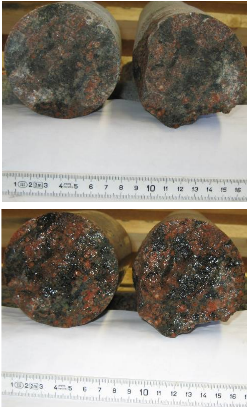
Figure 5–31. The fracture surface for the fracture at 0.199 m in the core. Dry and wet surface.
