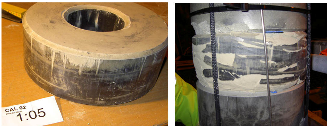
Figure 21. Left: A Calcigel block prior installation (block 1:05). Right: The same Calcigel block as to the left is showing damages shortly after the completion of the first package assembly. The surface was fractured and pieces had fallen off the block.
