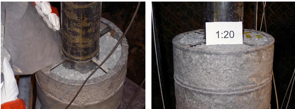
Figure 16. The cage is filled with granulate, left. A completed cage to the right.
