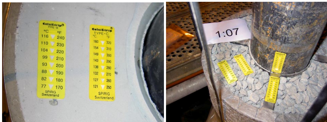
Figure 9. Left: Temperature indicators in position on a buffer block. Two different ranges are used on the sensors. 77 to 116°C and 121 to 160°C. The higher range indicator is located closer to the heater pipe. Right: Indicators are also placed on the frame of the granulate holding cage as well as on the granulate.
