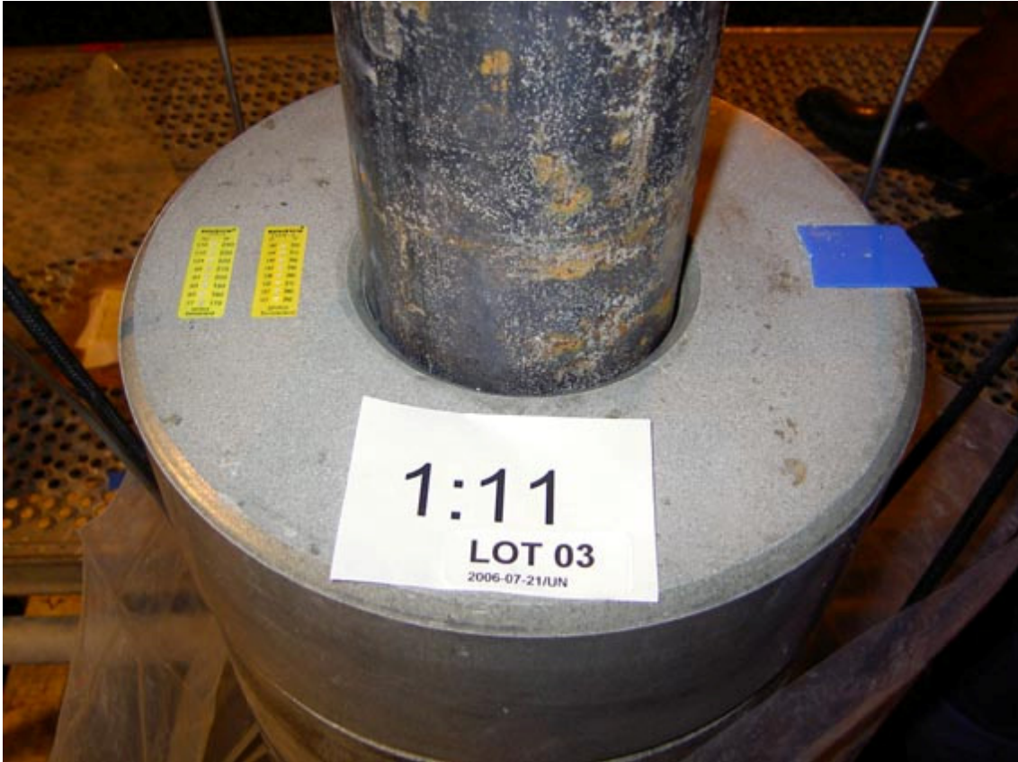
Figure 15. A small blue plastic plate is placed between each block, to the right in the image This will help identify the blocks during the package disassembly. The picture shows the eleventh block in the first experiment package, this is a MX80 block (ID code LOT 03). To the left the two temperature indicators can be seen.
