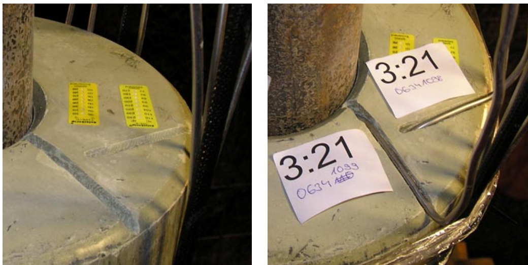
Figure 5. Installation of thermocouple sensors. The left image shows the notches made to house the sensor shields. In the right image two sensors are installed. (The code 3:21 represents package 3, block 21.) The yellow stickers are temperature indicators, described in section 6.3.
