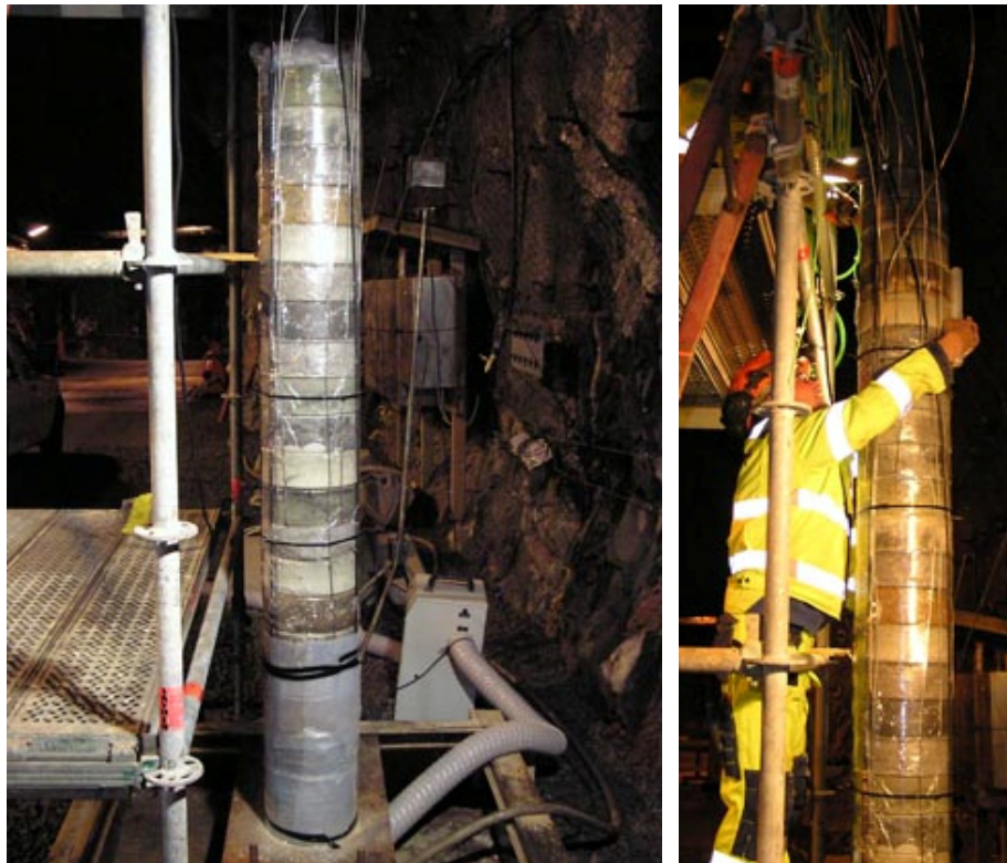
Figure 17. Left: Package two thirds finished, wrapped in plastic. Right: Finalizing the second package assembly with sensors cable aligning and plastic wrapping.
