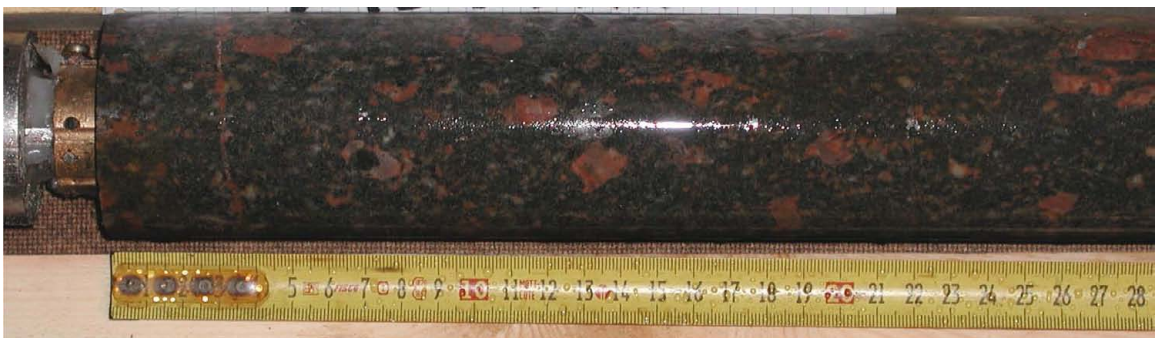
Figure G1. Photos of pilot core and overcore sample for borehole KQ0061G10.
