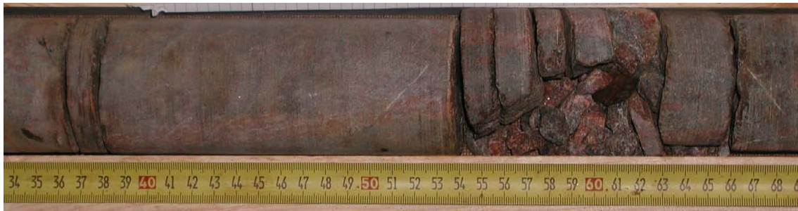
Figure 4-2. Observed core diking in borehole KQ0062G06 at 0.56–0.64 m depth.
