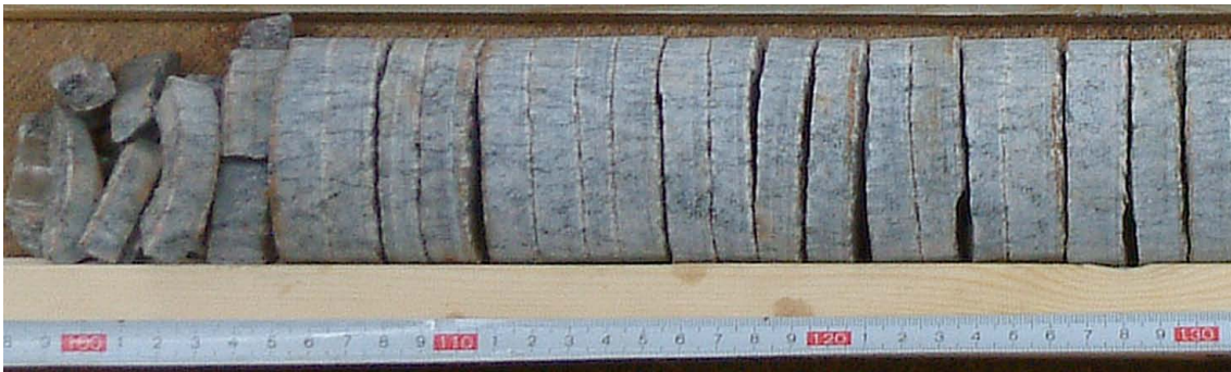
Figure 1-1. Example of ring disking observed during overcoring rock stress measurements in borehole KFM01B (test no. 2:10:1 at 474.25 m depth) /Lindfors et al., 2005/.
