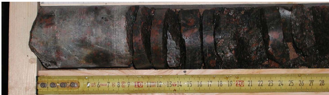
Figure 4-3. Observed core diking in borehole KQ0062G06 at 2.51–2.67 m depth.
