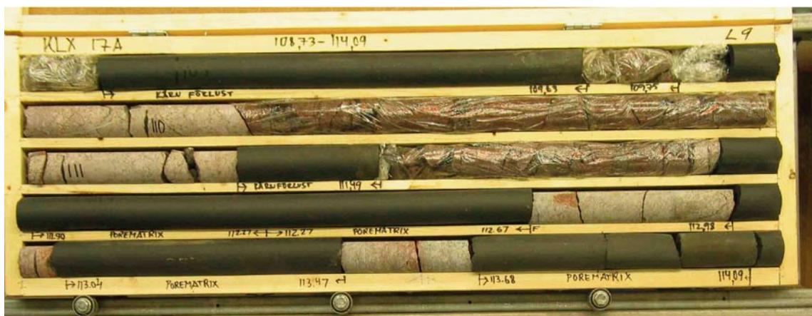
Figure 5-10. Core box from KLX17A with removed portions of core for pore matrix sampling (111.90 metre and below). Two sections with core losses are also noted at 108.70 and 111.23 m.
