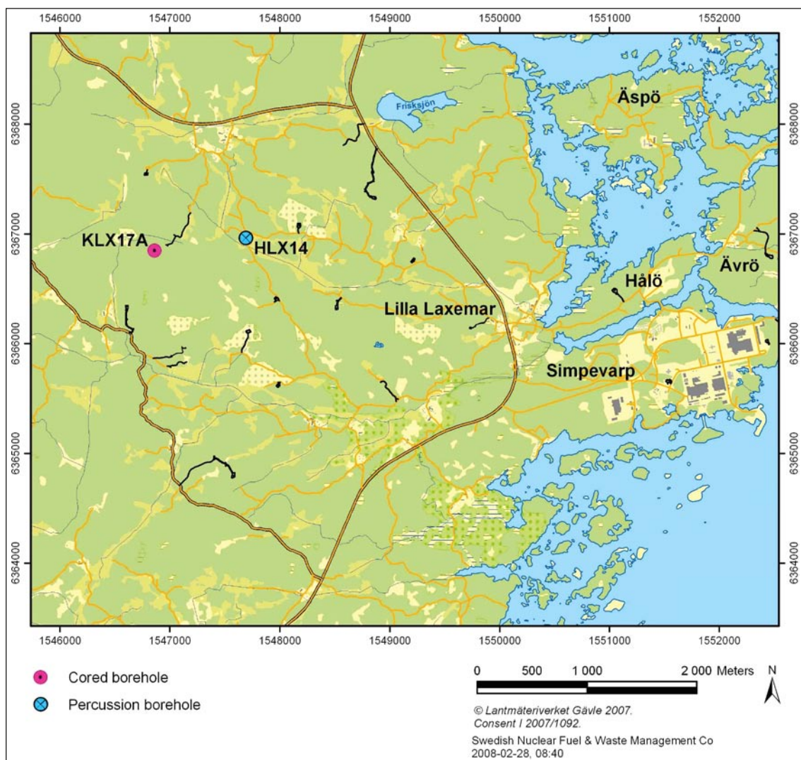
Figure 1-1. Location of the cored borehole KLX17A and the water source, percussion borehole HLX14 in the Laxemar subarea.
