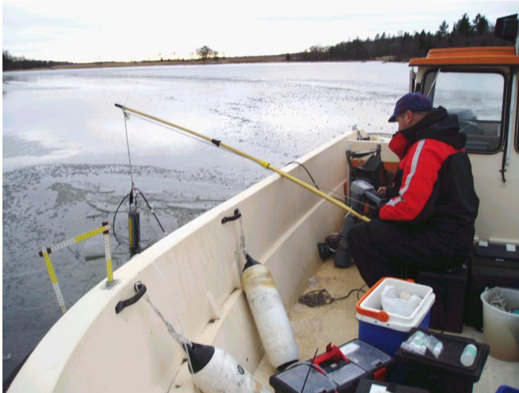
Figure 5-1. Measuring a profile (PFM000064) in the ice covered Baltic Sea with the multiple sonde (YSI 6600 EDS).
