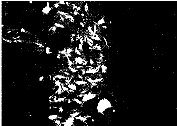
Plate I-16. BSEM photomicrograph showing fine-grained fibrous chromium ettringite (bright) replacing part of the cellular fabric of woody plant material reacted with hyperalkaline groundwater. Sample C364, Fluvial Boulder Gravel, Western Springs, Maqarin.
