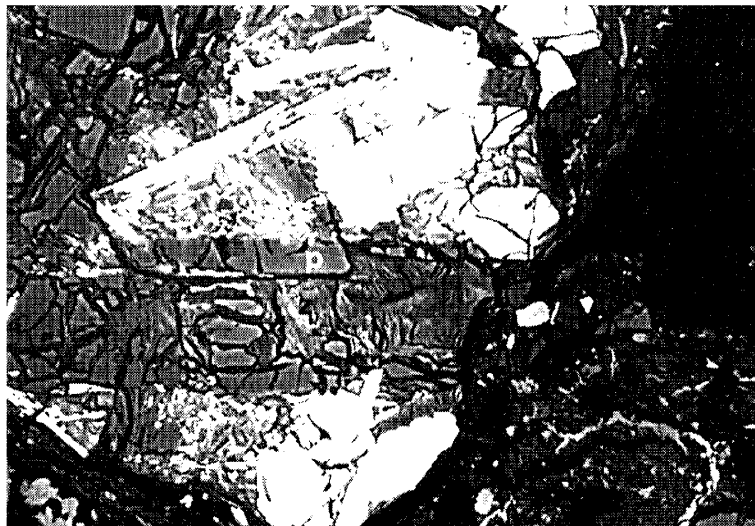
Plate I-8. BSEM photomicrograph showing highly altered plagioclase (p) at the margin of a basalt clast which is largely altered to secondary amorphous or gel-like CASH (z). Sample C362, Fluvial Boulder Gravel, Western Springs, Maqarin.
