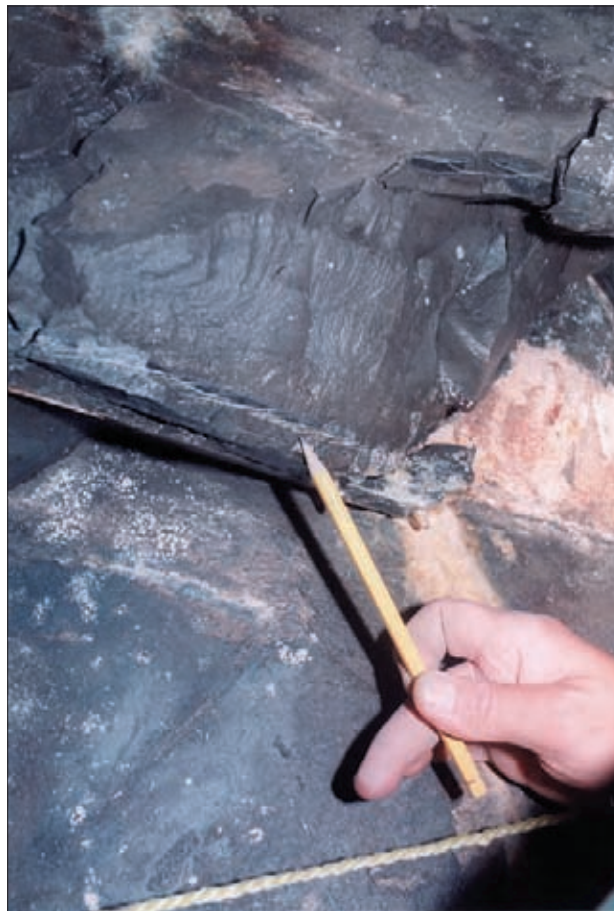
Figure 2-9b. Bedding plane parallel shear zone in a N-E dipping bedding plane at sampling site M2, Adit A-6. Note otherwise massive nature of the Bituminous Marl Formation (from Alexander and Mazurek, 1996).
