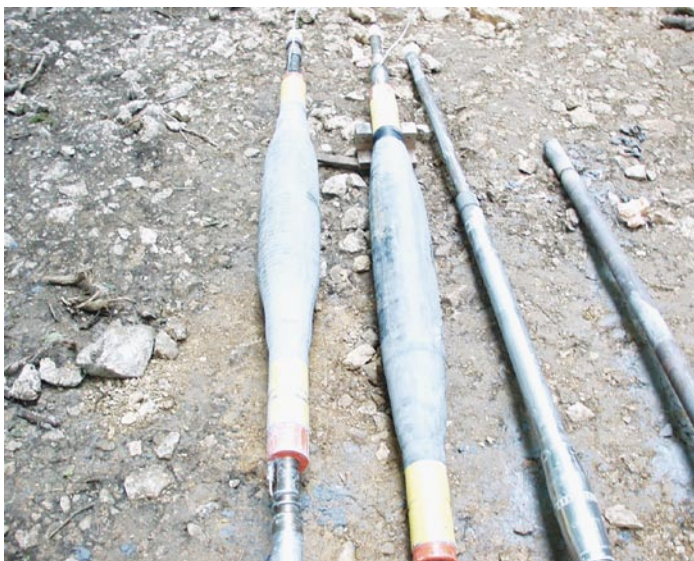
Figure 3-3. The straddled packer system showing its large deformability implying that it may operate in wells with variable diameters.
