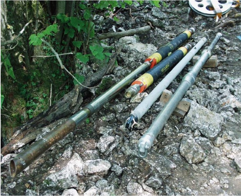
Figure 3-4. The straddle packer and the HTPF tool. The top of the downhole assembly is shown in the lower, left corner and terminates with the upper packer element. The second and third parts include the lower packer element and a weight used in inclined boreholes (mounted below the HTPF tool), respectively. The fourth part is the HTPF tool where the thicker central part contains the electrodes.
