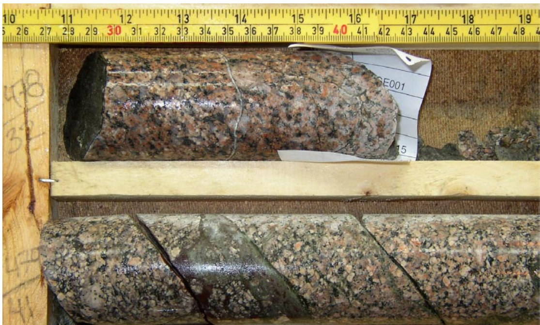
Figure 5-46. DZ 7. Uppermost transition zone, with gently dipping open fractures and a discrete olive-green ultracataclastic band.
