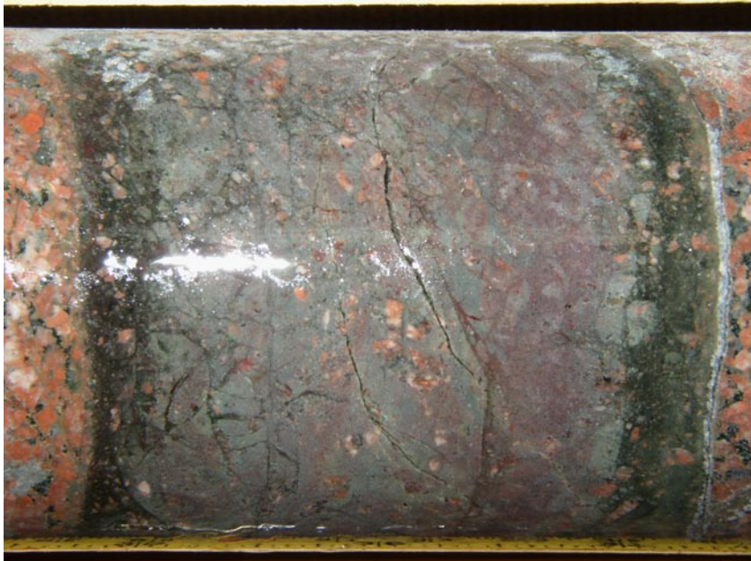
Figure 5-117. DZ core, extending from 378.795 to 378.850 m depth. The core consists of cataclasites and ultracataclasites with differently coloured matrix. The outer rim of the core has a dark green colour and contains fragments of the granitic host rock. The ultracataclasite with the greyish-green matrix contains fragments of a previously formed and indurated cataclasite and clasts of the hosting granite, while the purple coloured ultracataclasite also contains fragments of the greyish-green ultracataclasite.
