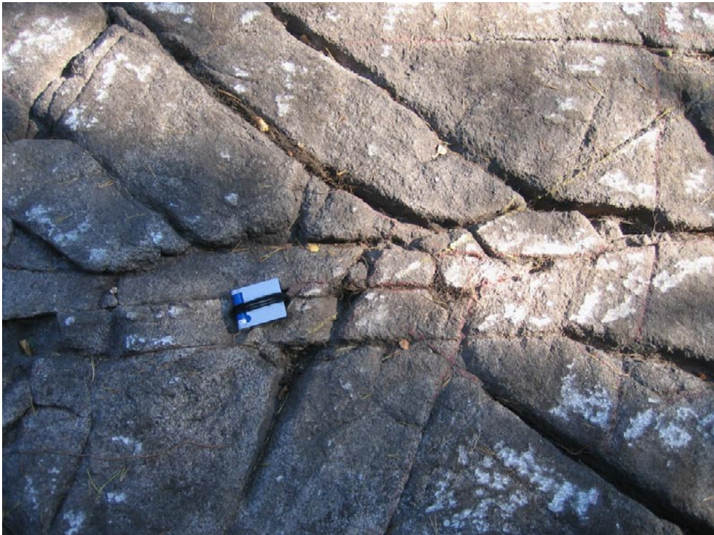
Figure 6-10. Example of complex fracture pattern, which does not allow the establishment of the relative timing of fracture formation, their hierarchy nor their kinematics.
