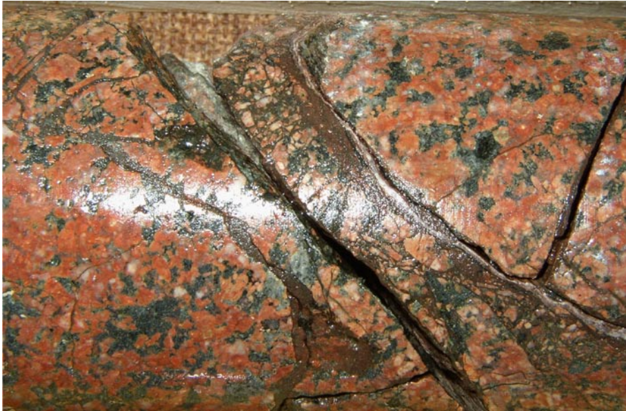
Figure 5-73. Detail of the network of proto-, ultra-cataclasites and gouge bands in the core of DZ 7 of KLX11A. Mechanical comminution has generated extremely fine-grained clasts. The cataclastic band is oriented 259/63.
