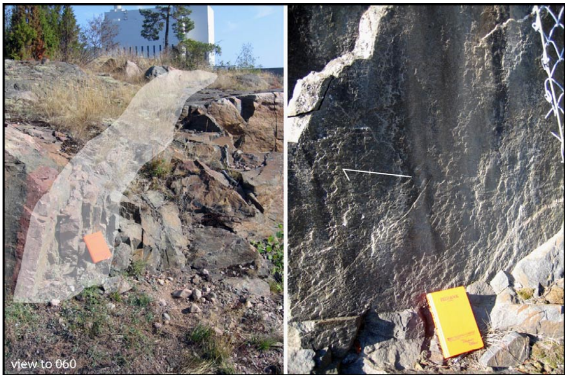
Figure 6-19. Left: the shaded white area highlights the width and the trend of the protomylonitic shear zone that dissects outcrop PSM007665 and whose orientation is shown by red great circles in Figure 6-18. In the background is visible Block 3 of the atomic power plant. Right: detail of the striated dextral fault oriented 345/84.
