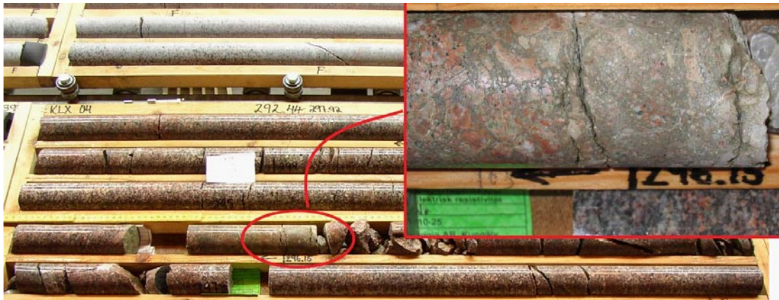
Figure 5-33. Overview of DZ 3 in KLX04. The red oval highlights the position of part of the cataclastic core of the deformation zone, a detail of which is shown in the inset. The core is strongly cataclastic and is rich in green ultracataclasites/gouge.
