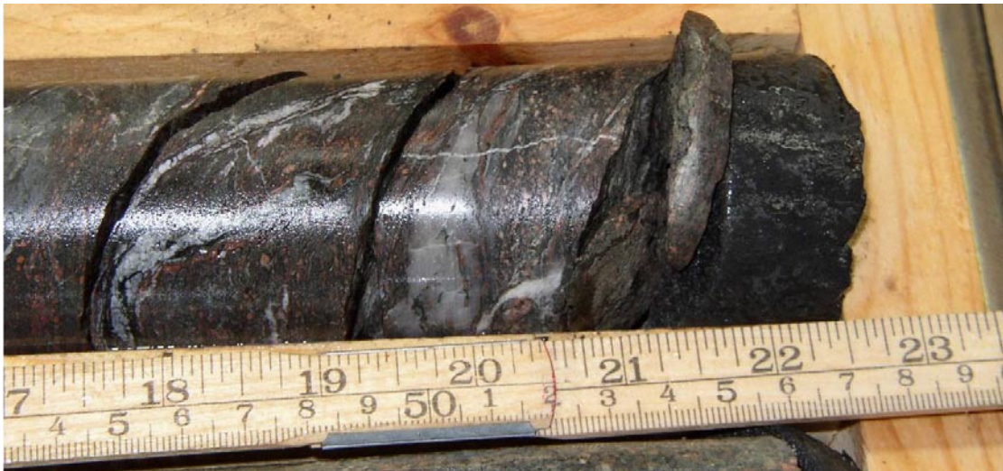
Figure 5-15. Foliated cataclastic quartz monzodiorites form the core of this very gently SW-dipping deformation zone core at depth 797–798 m.
