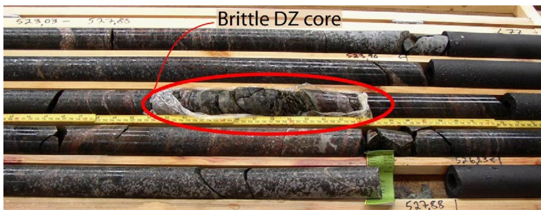
Figure 5-81. Highly fractured brittle core in DZ 12. The core is located in a pervasively foliated quartz monzodiorite.
