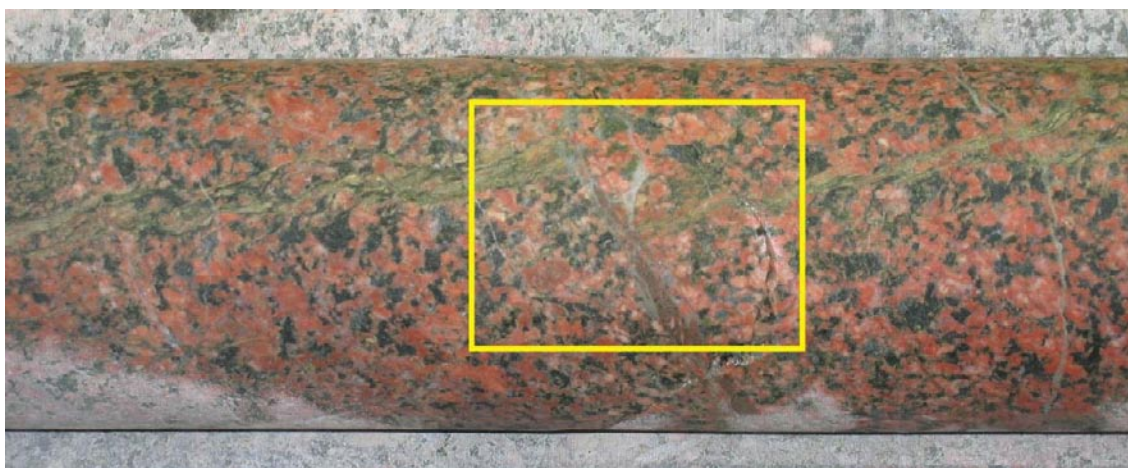
Figure 5-19. An epidote-decorated brittle ductile shear zone is offset along a flatter discrete brittle fault at depth 806 m.
