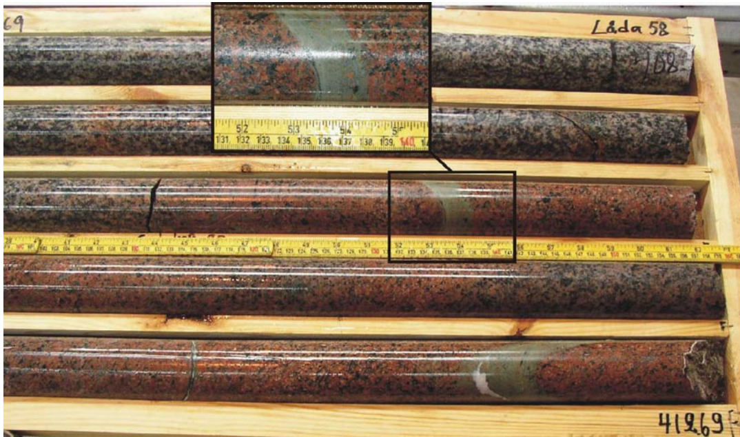
Figure 5-134. DZ 4 consists of relatively undeformed rock with only a few epidote-calcite dilatant bands.
