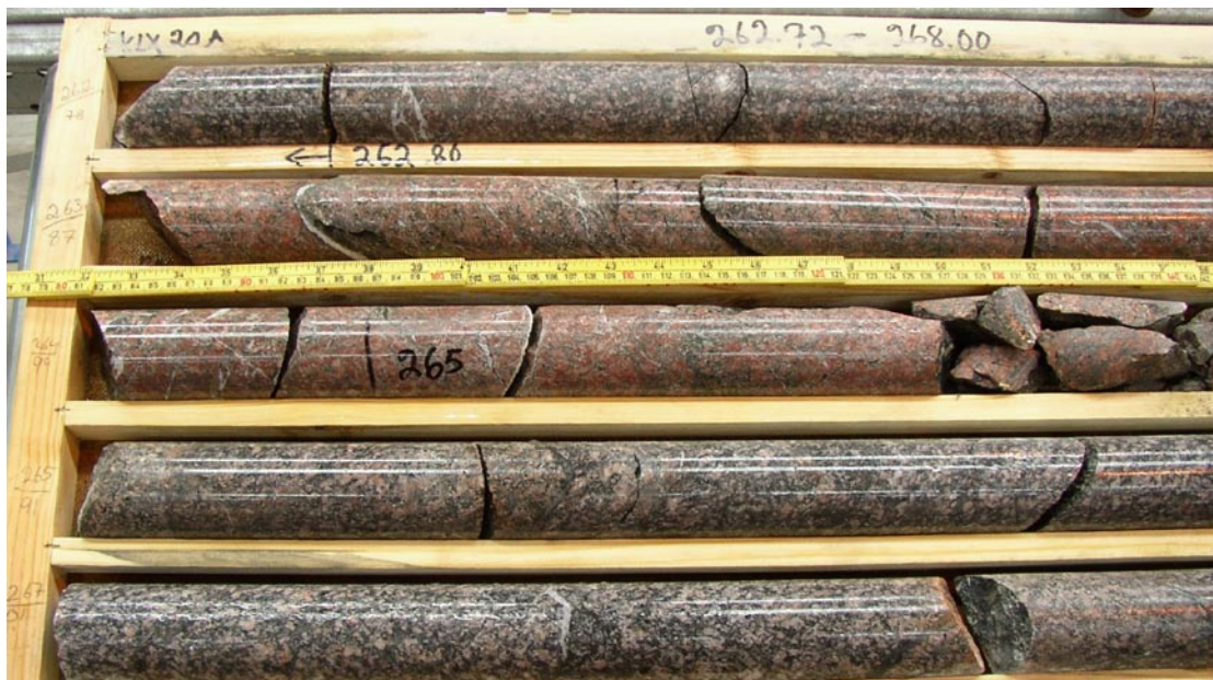
Figure 5-132. DZ 2 consists of relative undeformed rock with only a minor crush zone.
