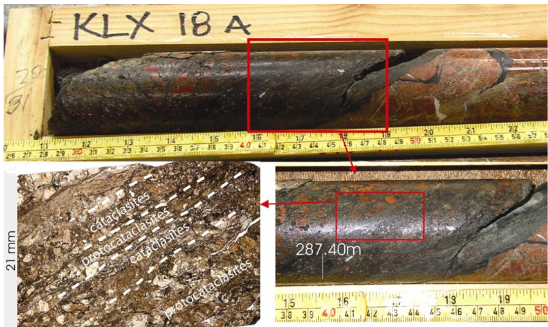
Figure 5-113. Sample KLY18-1 from cataclastic granites at depth 287.4 m. The scanned thin section shows a faint foliation within the sample (white dashed lines), which is defined by the alternation of protocataclastic and cataclastic domains.
