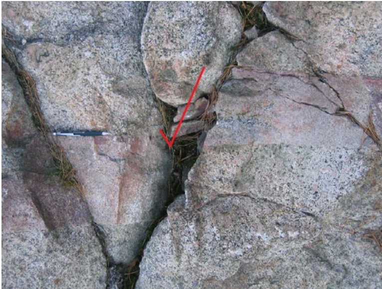
Figure 6-16. Sinistral displacement of a granitic dyke across a fracture of set Y.
