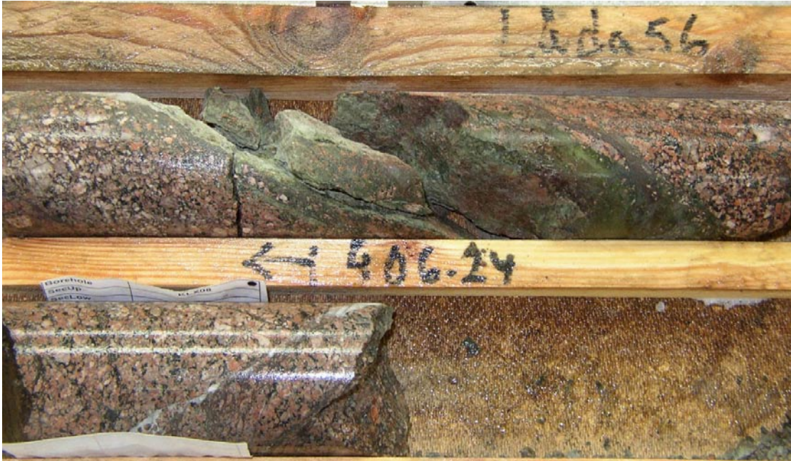
Figure 5-43. Epidote ultracataclasite at depth 406.18 m. The ultracataclasite and the open fracture are oriented 150/41.
