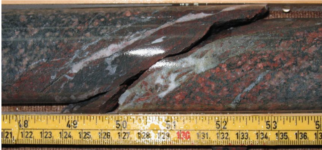
Figure 5-92. A broken fracture, coated by calcite, epidote and clay minerals and oriented 180/87, follows a dilational calcite epidote vein and exploits a pre-existing protocataclastic band. A faint foliation is visible, suggesting deformation at the brittle-ductile transition.
