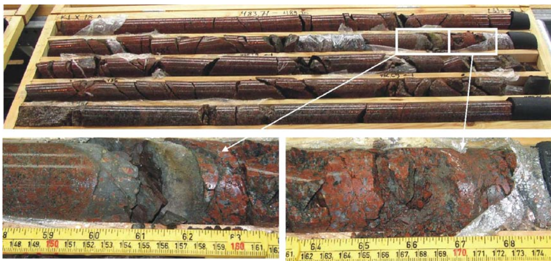
Figure 5-124. DZ 9 is characterized by an upper transition zone extending from 471.9 to 488.9 m depth, which is defined by a progressive increase of the fracture frequency (upper photograph, two upper rows before the white boxes). The core (details shown in the two bottom pictures) consists of cataclasites, a gouge interval and a strongly fractured rock interval.
