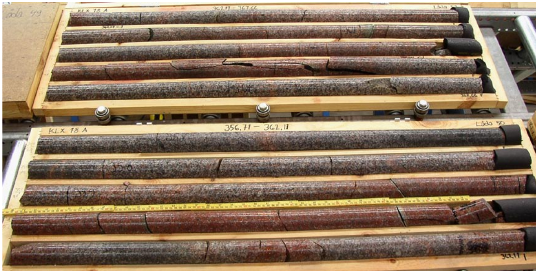
Figure 5-115. DZ 4 359.6–366.2 m (Box number 50 and 51). This DZ consists of moderately to little fractured rock with localized red staining. The bedrock is Ävrö granite.
