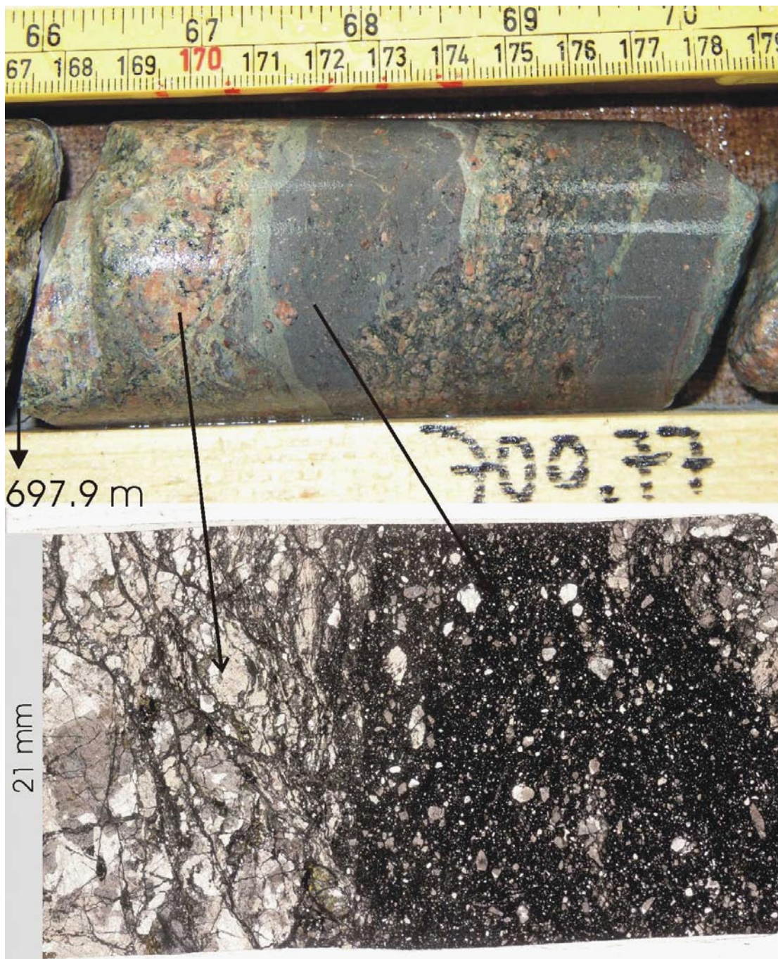
Figure 5-63. Sample KLX10-1 from depth 697.9 m illustrates the existence of several generations of cataclasites and ultracataclasites, with the fine-grained (grey) ultracataclasite containing fragments of “older” cataclasites in turn formed at the expense of the hosting granite. The black matrix in the thin section is extremely fine grained (hence the black colour) and is the equivalent to the grey-coloured matrix in the drill core. The transition from the cataclasite to the left to the ultracataclasite to the right is gradual and is the result of the progressive mechanical reworking of the protocataclasites.
