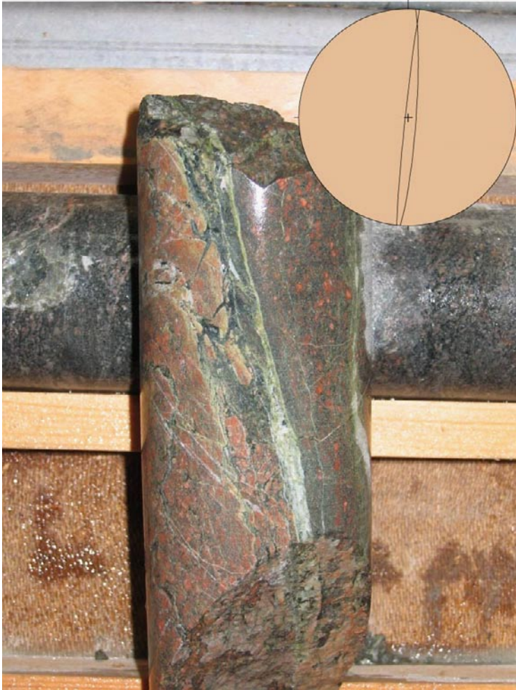
Figure 5-17. Steep, N-S trending fault with cataclasites and abundant epidote alteration. The stereonet plots the orientation of the structure.
