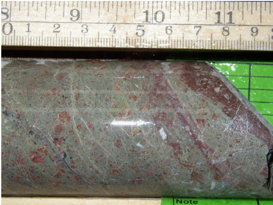
Figure 5-13. Detail of the lower part of the deformation zone central core. A brown ultracataclasite/gouge (to the right hand side) cuts across epidote-rich brecciated granites. Note the poor sorting of the clasts and their angular shapes.
