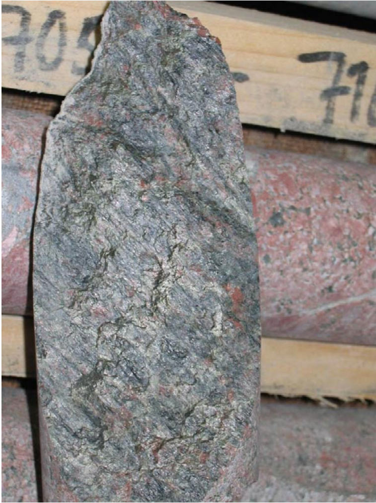
Figure 5-54. Example of a striated plane at depth 701.676 m. Chlorite, calcite and clay minerals coat the surface. Slickensides indicate that the hanging wall to this plane moved up parallel to the striations.
