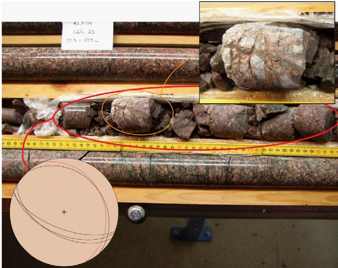
Figure 5-21. Brittle fault core and associated crush zone at depth 227.60 m in KLX04. The stereonet shows the orientation of selected fracture planes within the DZ core. The red great circle is the fracture oriented 337/26 at the base of the zone. Note the cataclastic texture of the core (inset on the top right-hand side) and the anastomosing sealed network of thin cataclastic and gouge bands in the lower transition zone immediately below the red oval.
