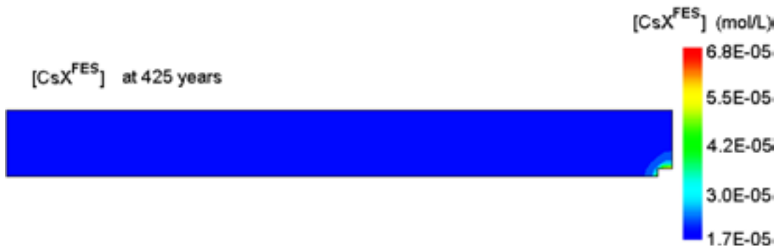
Figure 6-30. Concentration of caesium in the FES of the illite interlayer at the end of the 425-year simulation period. Only a very small area in the lower right corner is affected.
