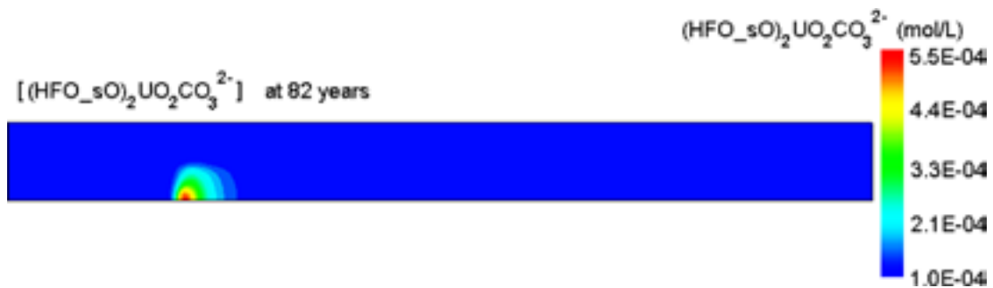
Figure 6-16. Predicted content of UO_2CO_3^{2-} adsorbed on the ferrihydrite surface ( \equiv(HFO\cdot O)_2UO_2CO_3^{2-} ) after 82 years.
