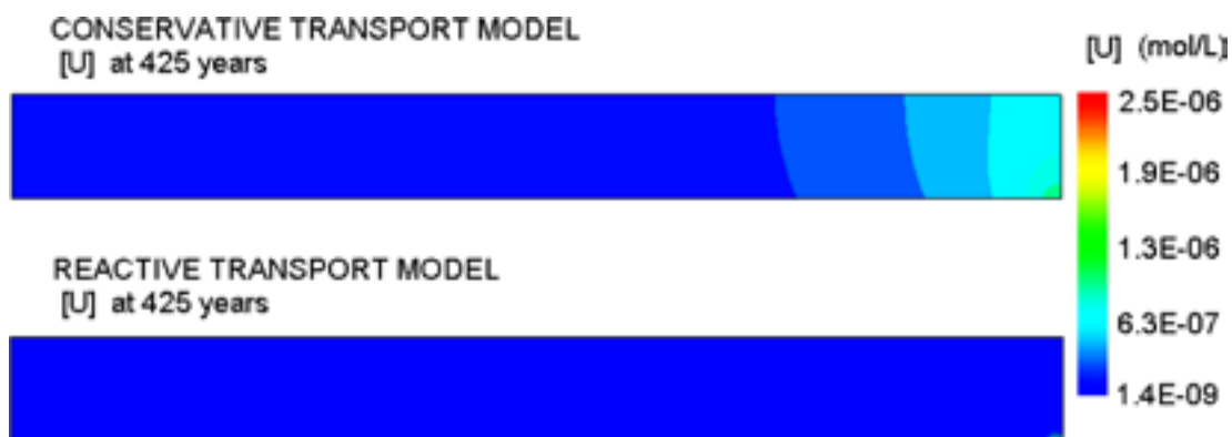
Figure 6-36. Spatial distribution of computed uranium concentration in the conservative simulation (up) and the reactive transport simulation (down), reference case #2 after 425 years. Only a very small area in the lower right corner is affected in the reactive transport case.
