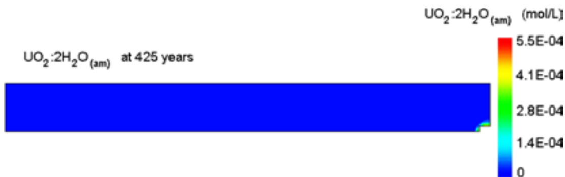
Figure 6-32. Concentration of UO_2 \cdot 2H_2O_{(am)} precipitated at the end of the 425-year simulation period.
