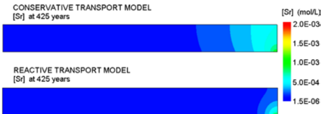
Figure 6-34. Spatial distributions of computed strontium concentration in the conservative simulation (top) and the reactive transport simulation (bottom), reference case #2 after 425 years.
