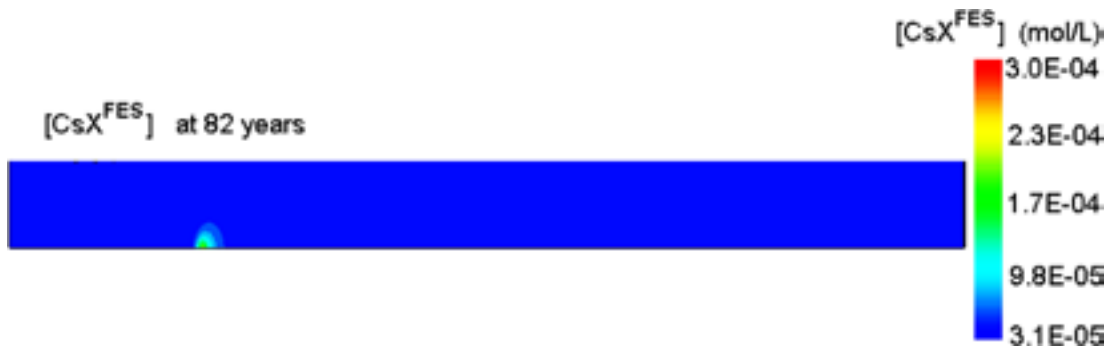
Figure 6-14. Concentration of Cs^+ in the FES, at the end of the simulation period (82 years).
