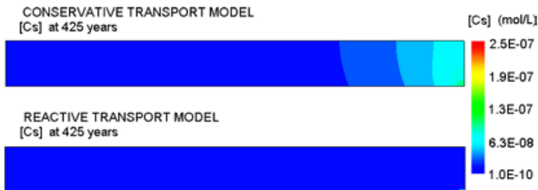
Figure 6-35. Spatial distribution of computed caesium concentration in the conservative simulation (top) and the reactive transport simulation (bottom), reference case #2 after 425 years. Only a very small area in the lower right corner is affected in the reactive transport case.
