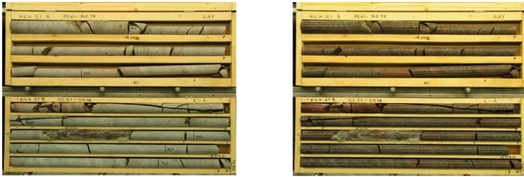
Figure 5-1. Core photographs of KLX21B, dry, 99–108 m and KLX21B, wet, 99–108 m showing a 4 row core box and a 5 row core box.
