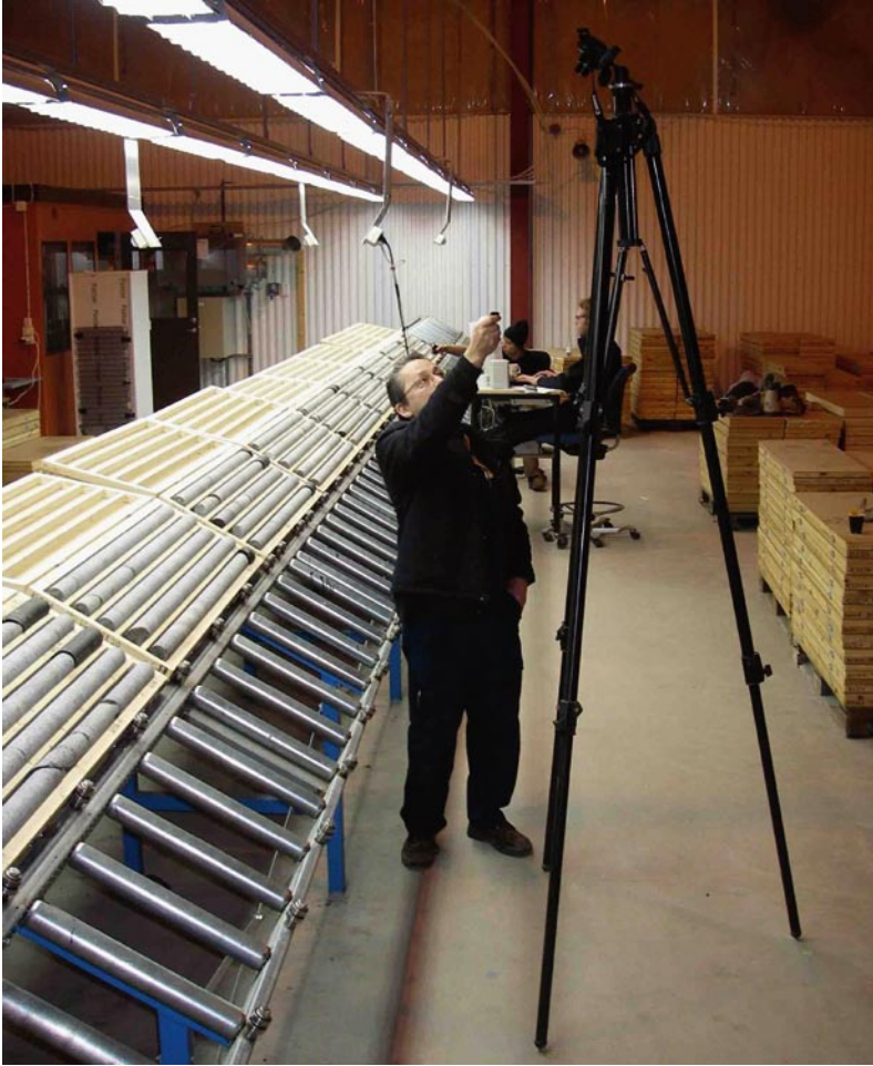
Figure 4-1. Photographing core in core boxes at the core shed in Simpevarp. Photographer is the person responsible for sampling and sample preparations Thomas Kiesel.
