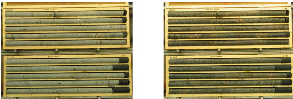
Figure 5-2. Core photographs of KLX19A, dry, 560–571 m and KLX19A, wet, 560–571 m showing 5 row core boxes.
