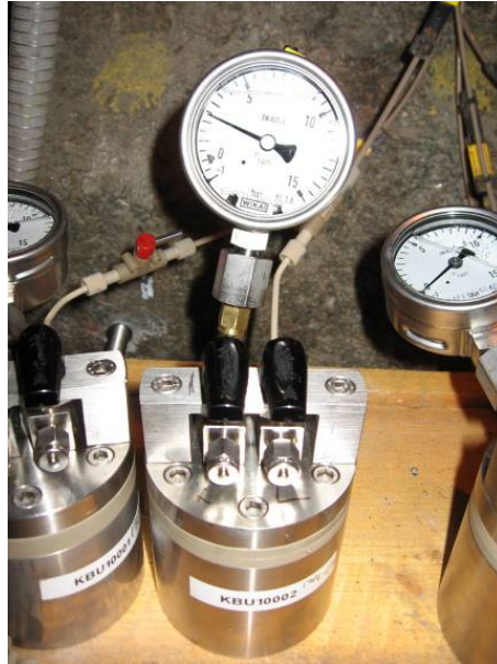
Figure 2-2. Pressure vessels used for extracting pore water and gas from the Prototype Repository.
