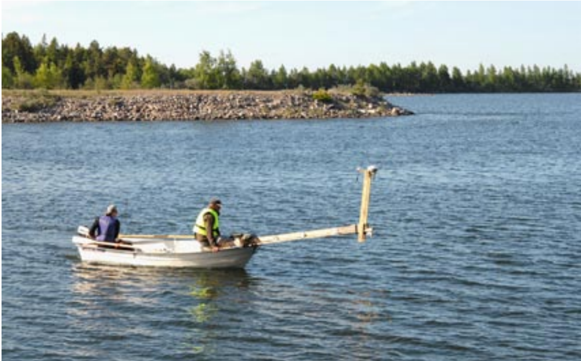
Figure 3-1. Magnetic seaborne survey on Asphällsfjärden using a small boat. The magnetic sensor is placed on a wooden frame in front of the boat, underneath the RTK-GPS-antenna. Photo: Alf Sevastik.
