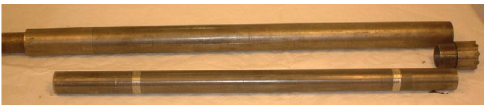
Figure 3-4. Bottom soil sampler was used.
