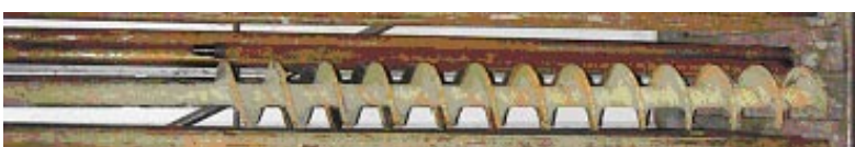
Figure 3-5. Soil sampling by auger drilling.
