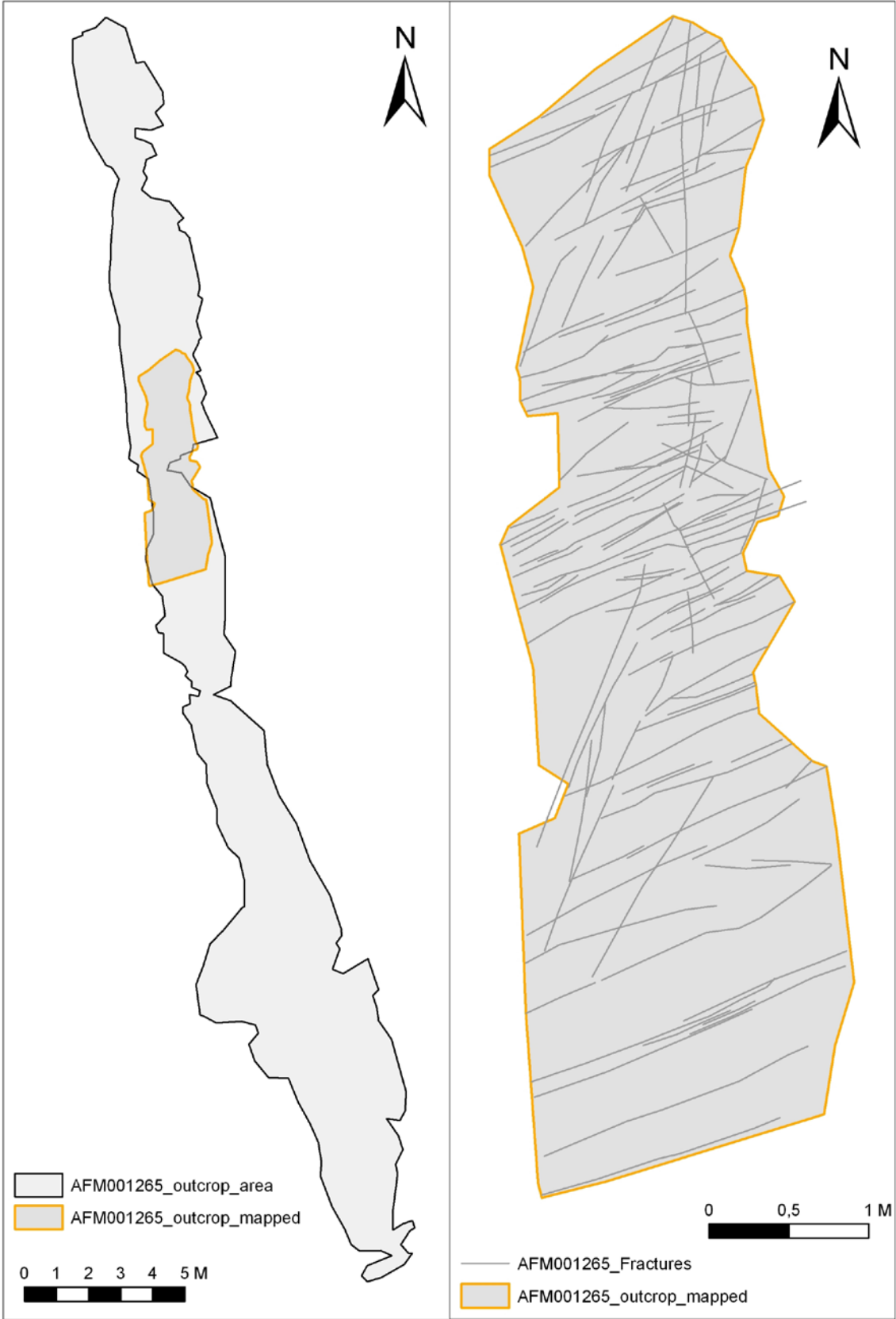
Figure 5-3. Fracture trace map of the fracture zone in the AFM001265 trench.
