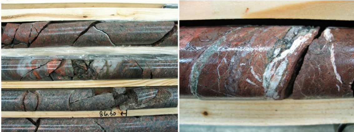
Figure 4-10. Deformation, ductile and brittle, as it appear at the probable location of the deformation zone MDZNS019A as it appears in KLX09D (left: c 85.5 metres and right: ca 88 metres core length).
