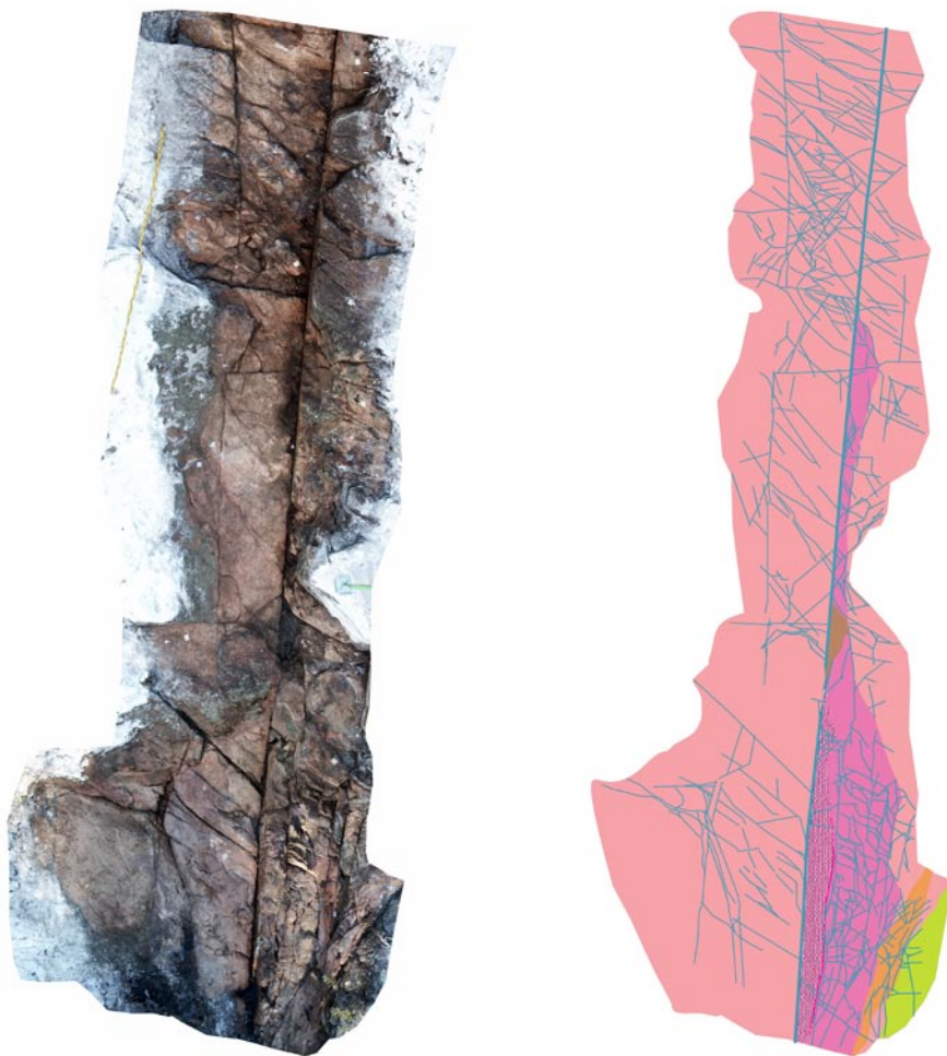
Figure 4-6. Example of documentation from the excavated zone MDZNS019A (North is upwards in the figure and the width of the outcrop is approximately 4 metres). On the left a high-resolution photographic image, that has been transformed to a close-range orthophoto. To the right a geologic map (schematic) showing fractures as blue lines and the rock types in different colours (pink = Ävrö granite, purple = fine-grained granite, orange = pegmatite, green = gabbro, brown = soil covered). A more intensely fractured part of the fine-grained granite is marked by a hatch pattern, bounded to the east by a fine-grained cataclastic rock (2 cm wide, dark purple in the figure).
