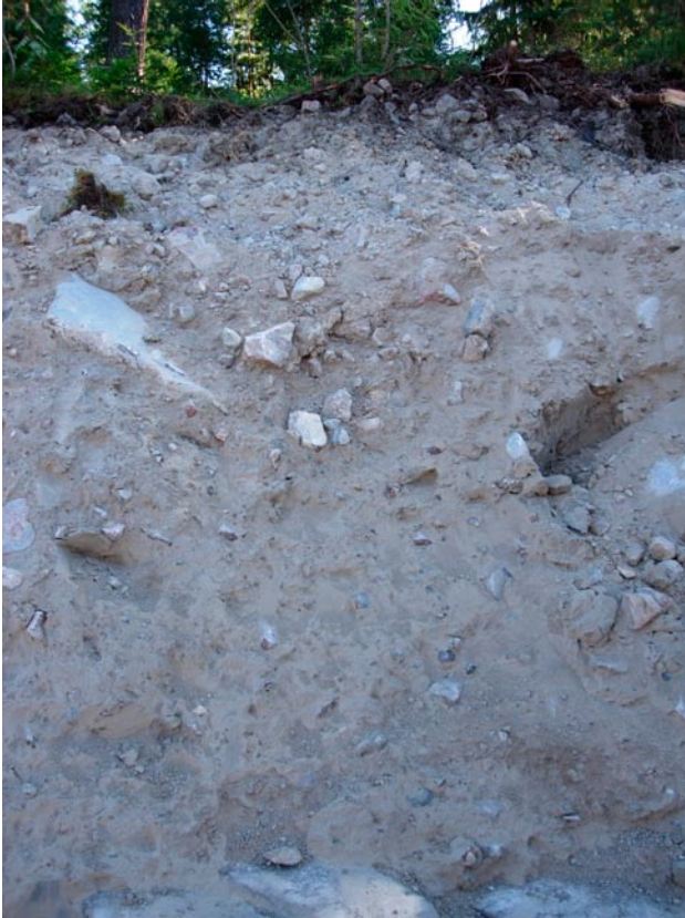
Figure B-7. Units 6 and 5 at PFM006614. Unit 6 appears dense and hard while unit 5 is sandy and loose.
