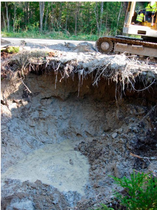
Figure B-10. High groundwater flow and unstable water saturated slopes prevented detailed investigations at site AFM001266.
