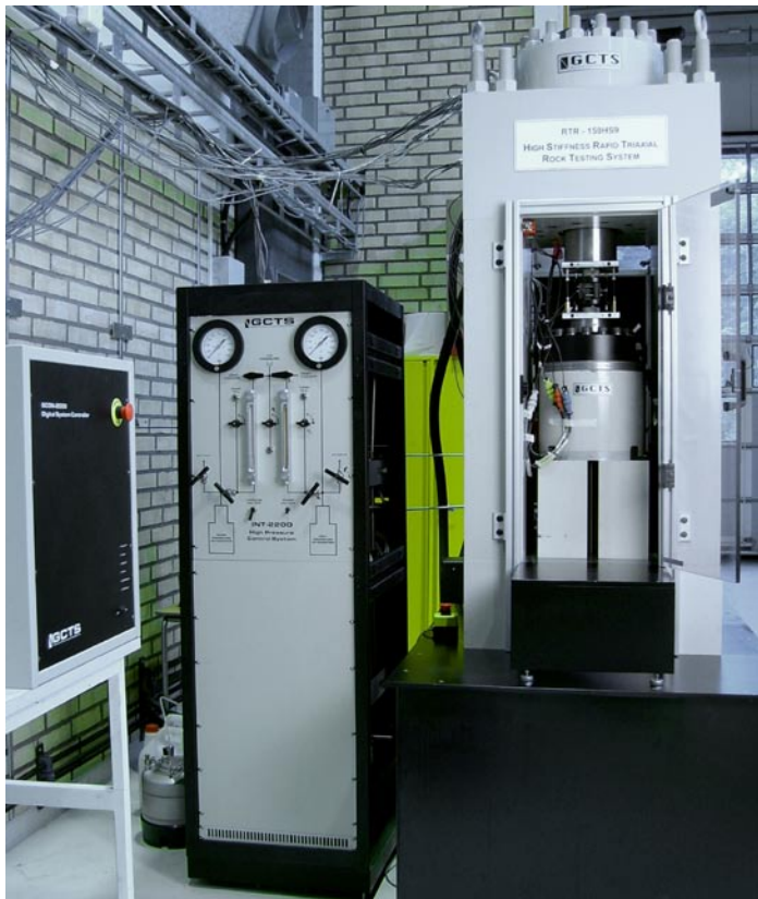
Figure 3-1. Rock testing system. From left: Digital controller unit, pressure cabinet (used for triaxial tests) and load frame. The PC with the test software (not shown in the picture) is placed on the left hand side of the controller unit.
