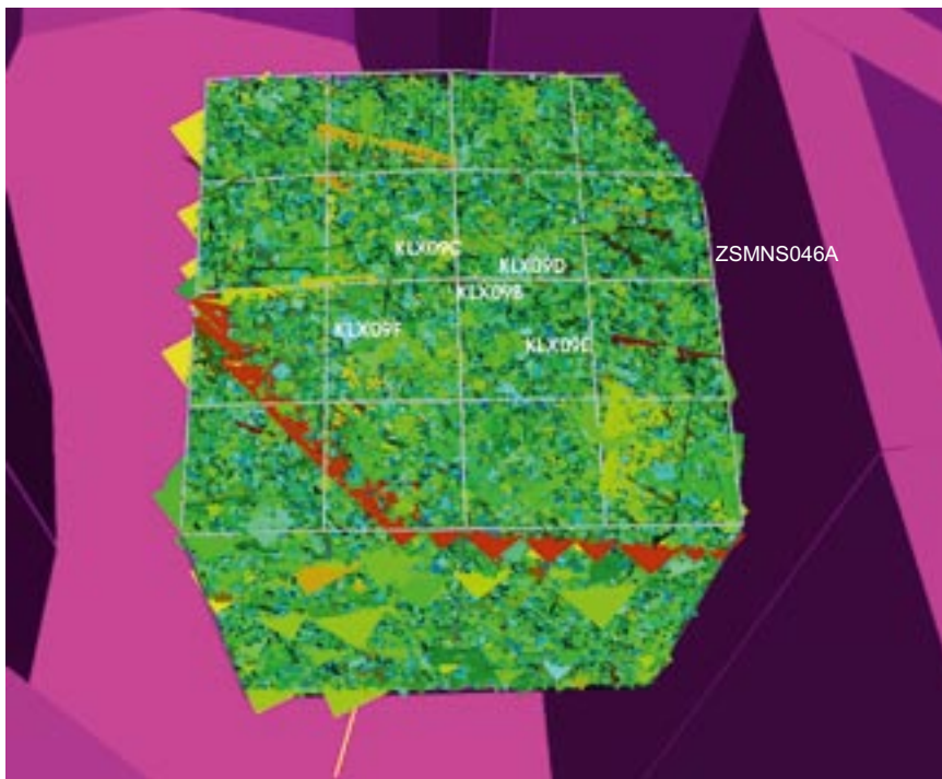
Figure 4-11. All fractures generated within the simulation domain and set in the context of the L 1.2 deformation zones. The fractures are coloured by \text{Log}_{10} transmissivity.
