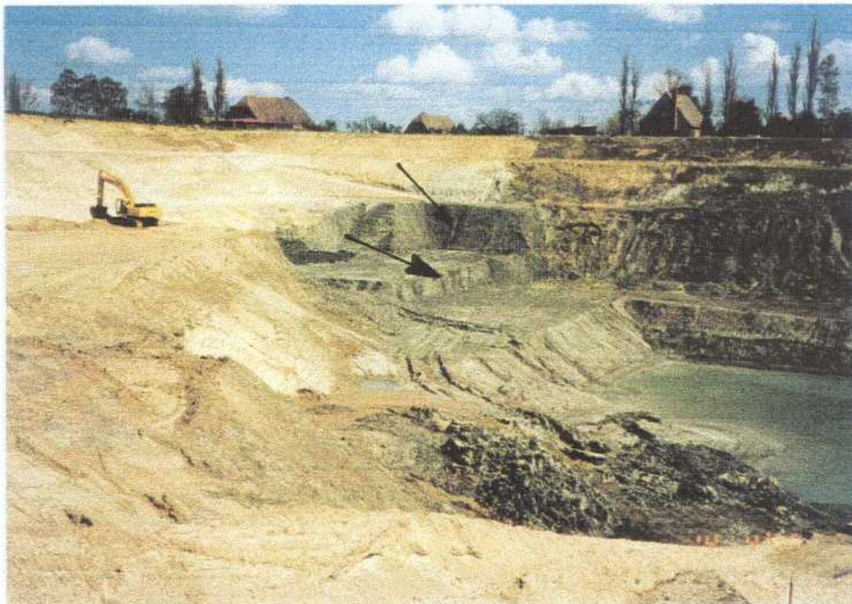
Figure 29. Photograph of the clay pit at Friedland. Arrows indicate slots excavated for taking samples.
