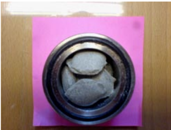
Figure 3-18. Pellet fill. Upper: Schematic picture of the microstructural constitution; the grains take up water from the boundaries by which they expand and give off clay particles that form gels in the voids between the expanded grains. Lower: Pellets with 10% water content in 30 mm cell.
