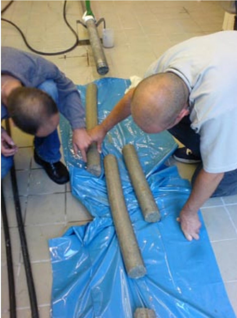
Figure 3-19. Appearance of the “Pellet” plug extruded from the tube used in the laboratory for the “piping” test. Notice the coherence of the plug which broke by mechanical strain at the expulsion.
