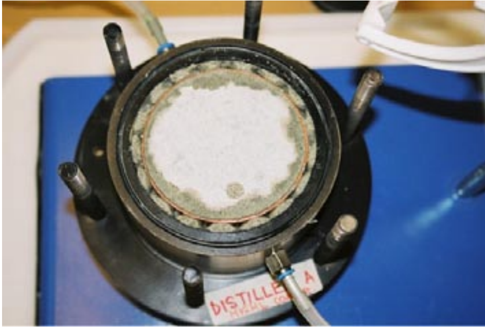
Figure 3-9. Growth of soft clay through the perforation of a copper tube confining a dense MX-80 clay core in an 80 mm diameter oedometer. Appearance at removal of the lid 8 hours after start. The larger part of the core is still unaffected by water.
