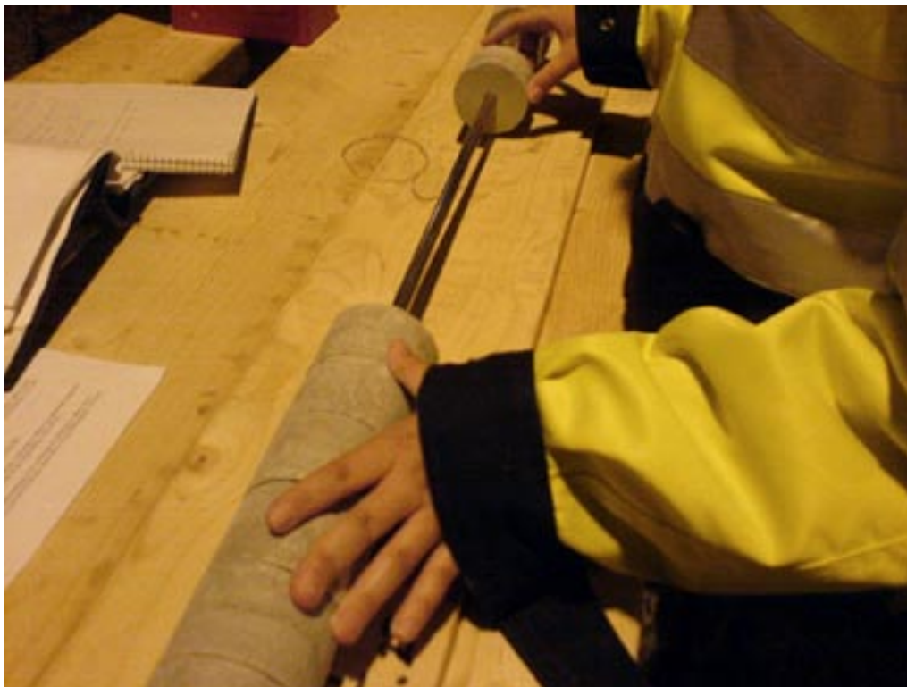
Figure 3-14. Preparation of the plug of Couronne type. The blocks are being stacked around the central rod.
