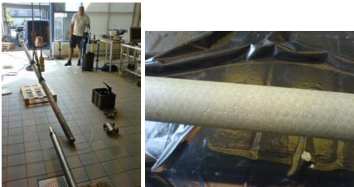
Figure 3-5. Left: The steel tube with the plug being exposed to a water pressure at the lower end. Right: Appearance of “Basic” plug extruded after 3 weeks of maturation under 500 kPa uniform water pressure /3/.
